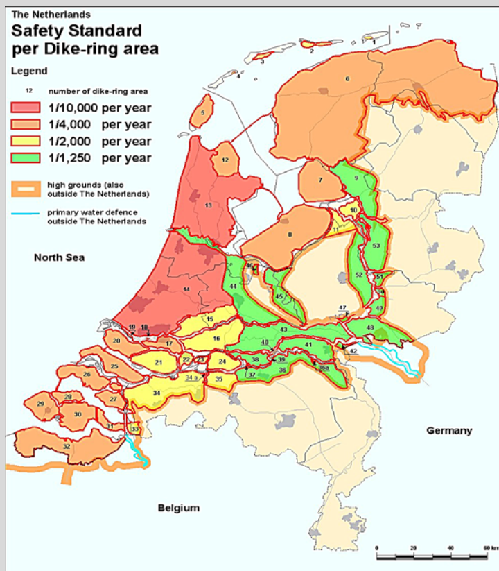
Figure A.1 Safety standards for primary flood defences in the Netherlands.
