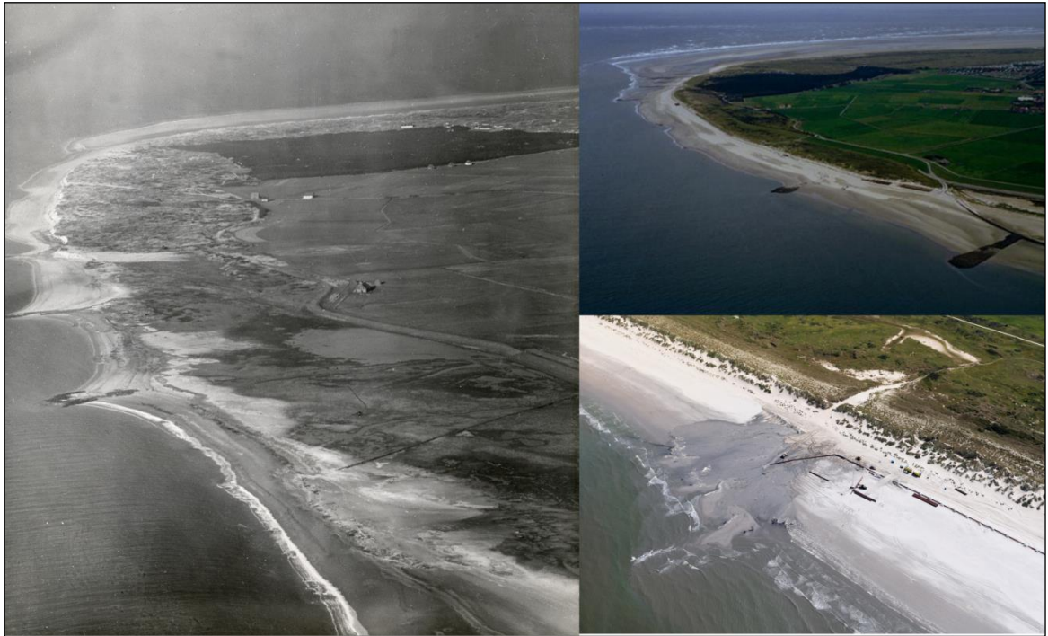
Figure 4.2 Impression of the coastal protection works along the west coast of Ameland ( https://beeldbank.rws.nl , Rijkswaterstaat). Left panel: Groins protecting the beach in 1954. Upper left: impression of the protection works in 2007, and (lower right) a nourishment taking place along the coast.
