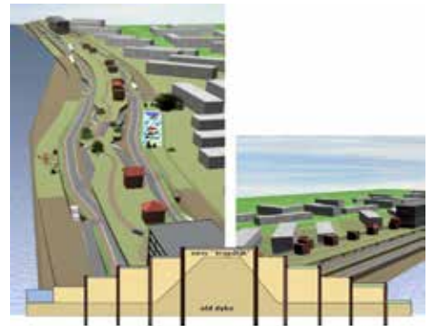
Figure 10: Step Dike, Rotterdam
