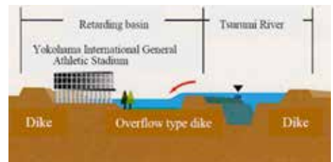
Figure 14: Location of the Yokohama stadium in the basin
