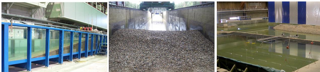
Figure 1. Applied small-scale (left) and large-scale (middle) wave flumes and multi-directional wave basin (right).
