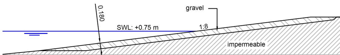
Figure 2. Model set-up in small-scale tests (for Series S1-S4).
