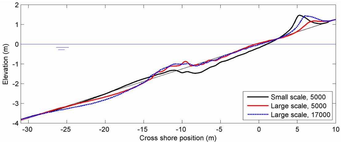
Figure 11. Comparison between large-scale and small-scale tests (with sand in pores).
