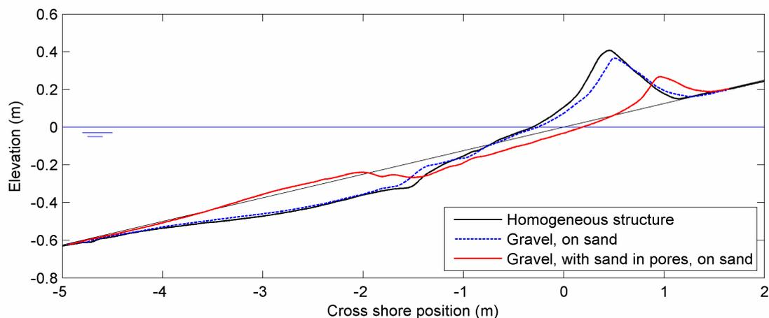
Figure 7. Small-scale tests: Influence of permeability.
