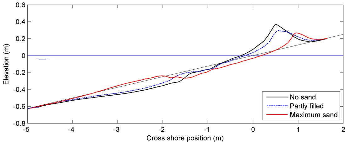
Figure 5. Small-scale tests: Comparison of profiles with and without sand in pores.
