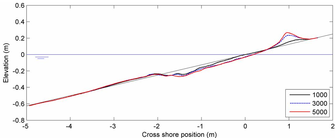
Figure 4. Small-scale tests: Development in time (with sand in pores).
