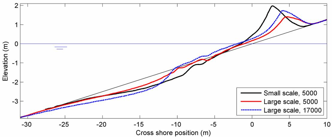
Figure 10. Comparison between large-scale and small-scale tests (no sand in pores).
