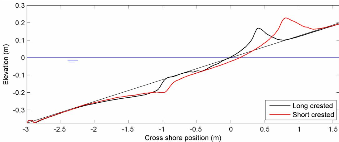
Figure 14. 3D tests: Comparison of profiles with long-crested and short-crested waves.
