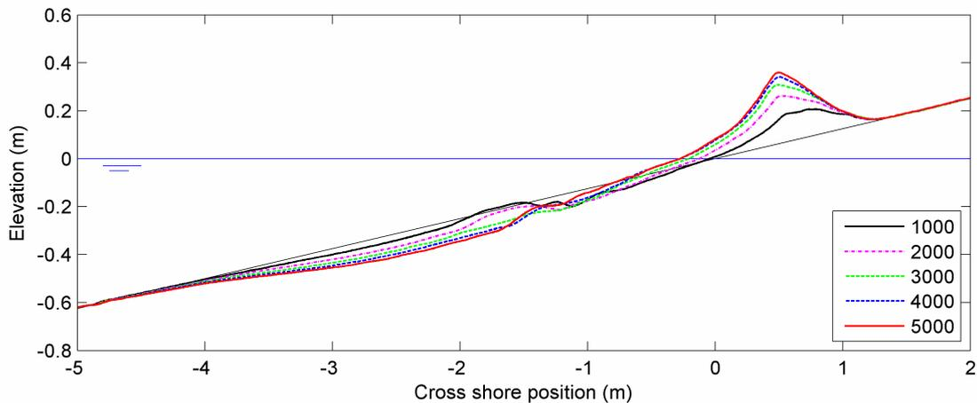
Figure 3. Small-scale tests: Development in time (no sand in pores).
