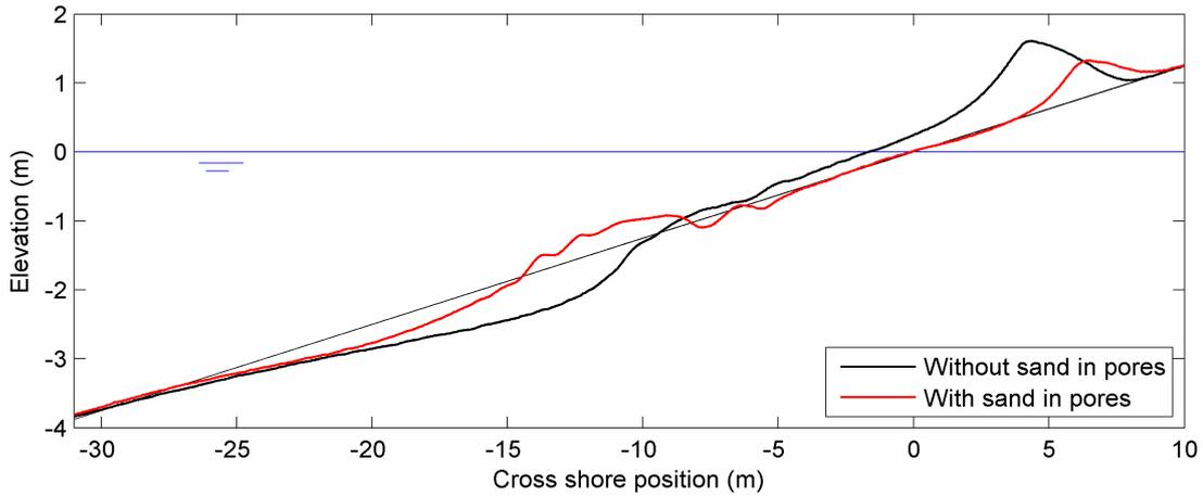
Figure 9. Large-scale tests: Comparison of profiles with and without sand in pores.
