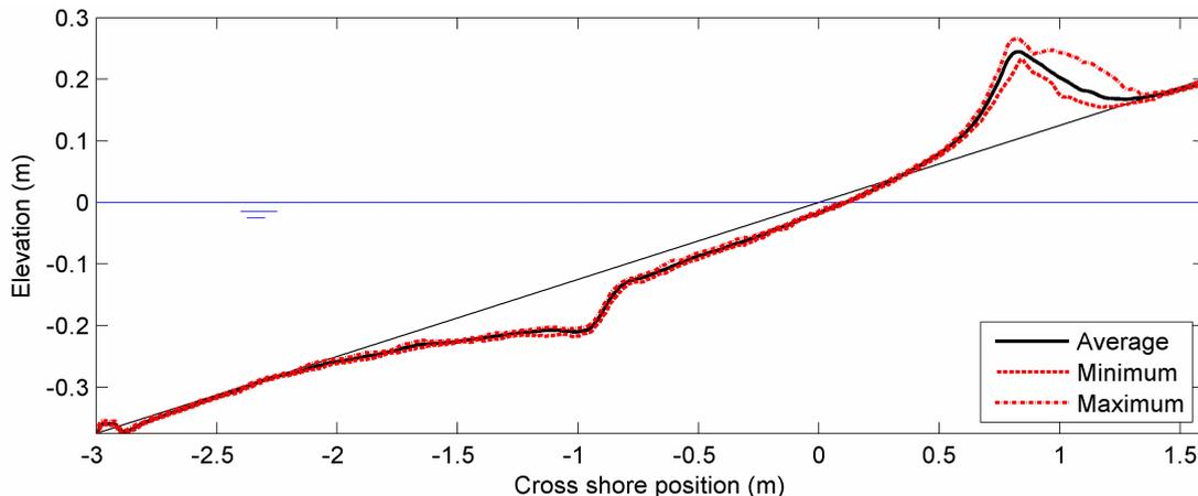
Figure 13. 3D tests: Differences between individually measured and average profile (short-crested waves).
