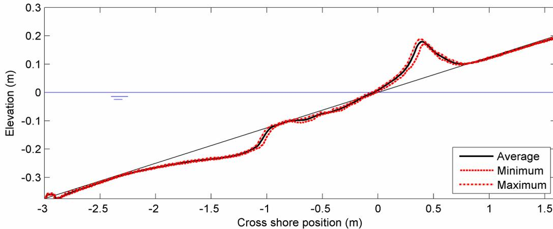
Figure 12. 3D tests: Differences between individually measured and average profile (long-crested waves).
