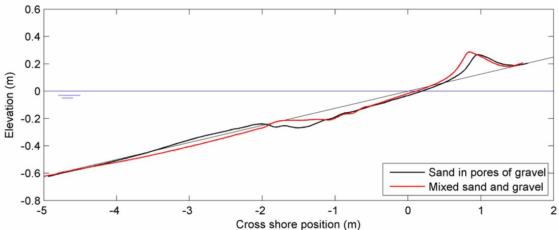
Figure 6. Small-scale tests: Comparison between profiles with sand in pores and a mixed beach.
