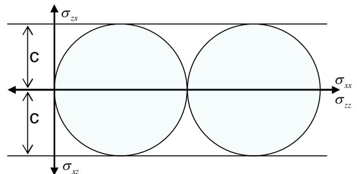
Figure 2: Mohr's circles to determine stresses under the footing
