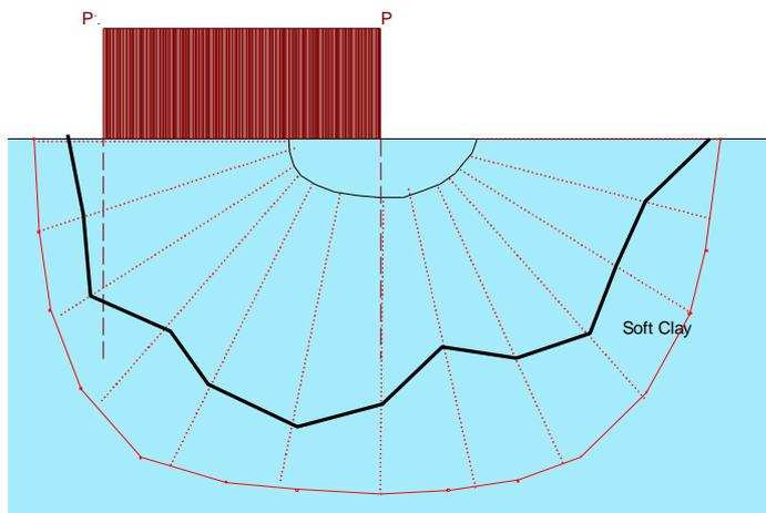
Figure 7: free definition of Spencer's slip plane
