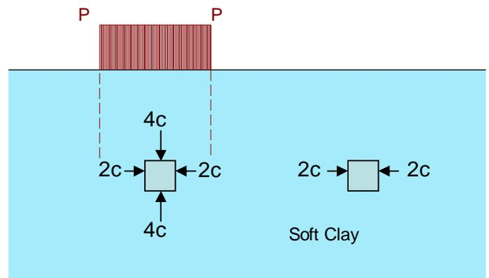
Figure 1: stresses underneath a strip footing
