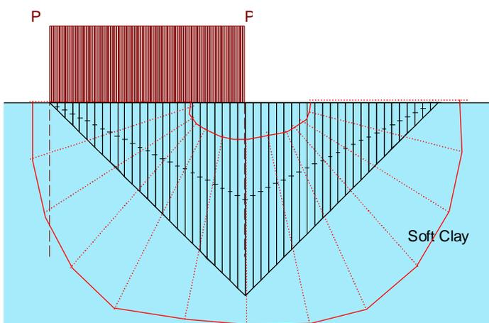
Figure 8: Upper bound by genetic algorithm with Spencer's method,  $f=4,00$
