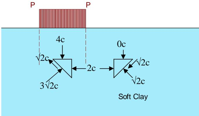
Figure 9: stresses underneath the strip load from figure 9
