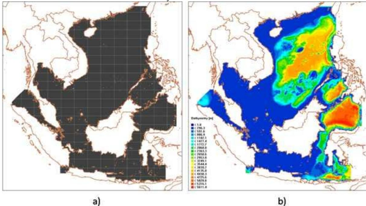
Fig. 3 Computational grid (a) and bathymetry schematization (b) of South China Sea Refined model
