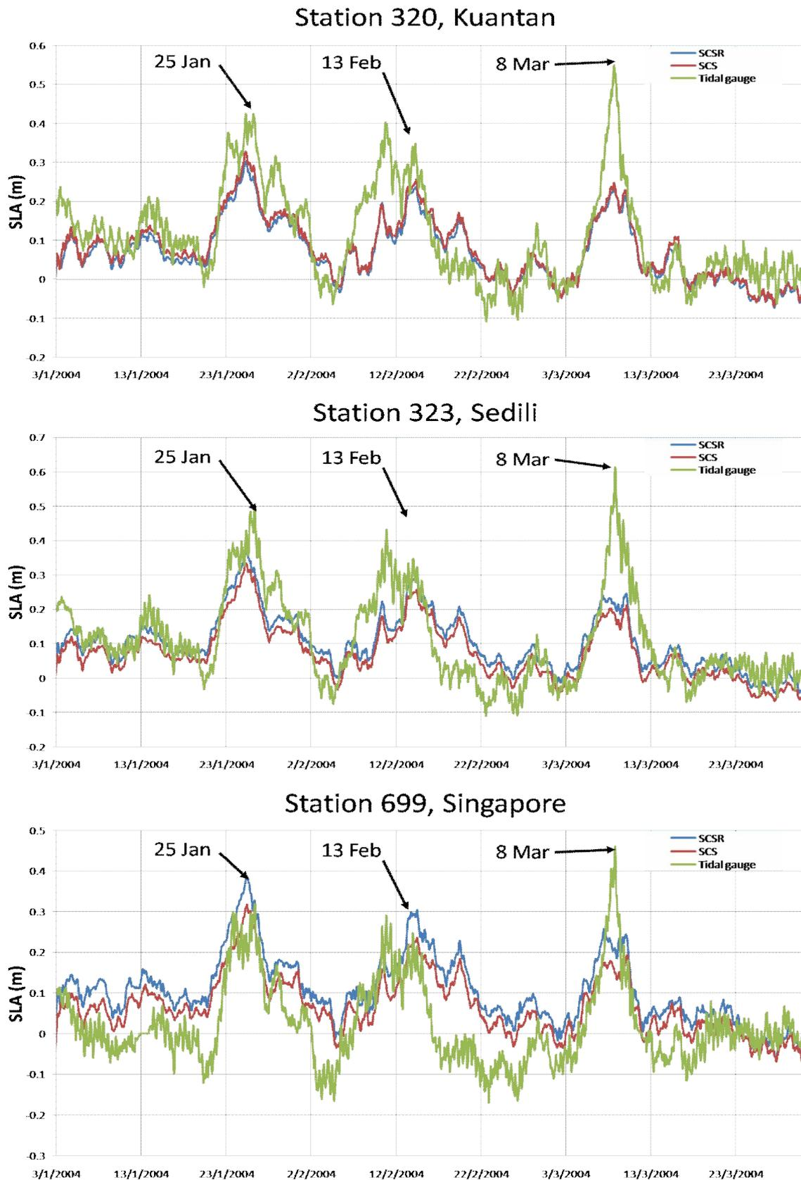
Fig. 4 Comparison between modeled and measured SLAs
