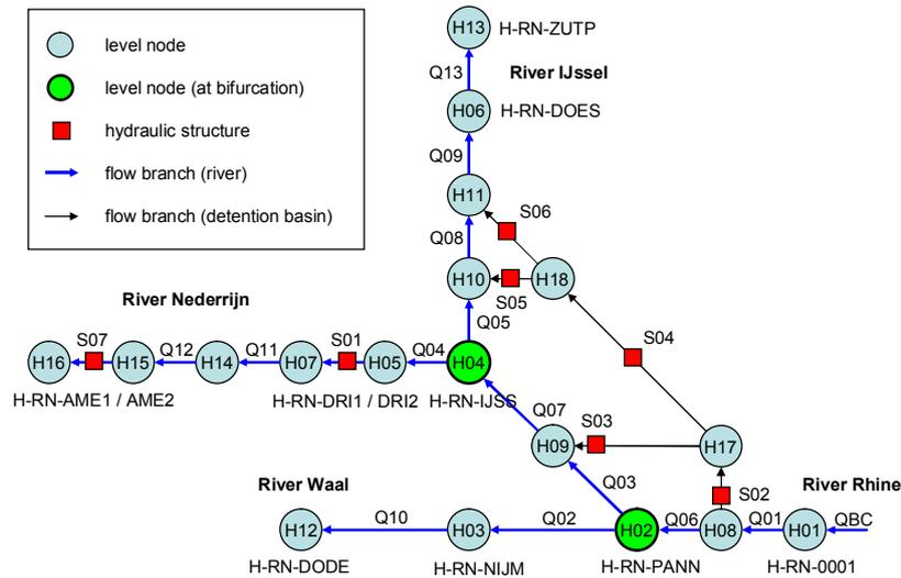
Figure 1 Layout of kinematic wave model: schematic overview about nodes and flow branches and hydraulic structure branches
