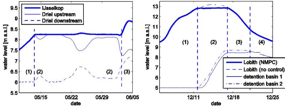
Figure 2 a) water level control at Driel during low - medium flow regime in May 2007 with water level set point of 8.25 m a.s.l. at gauge IJsselkop, b) damping of small flood peak above 12.75 m a.s.l. in December 2007 at gauge Lobith by control of detention basins 1 and 2
