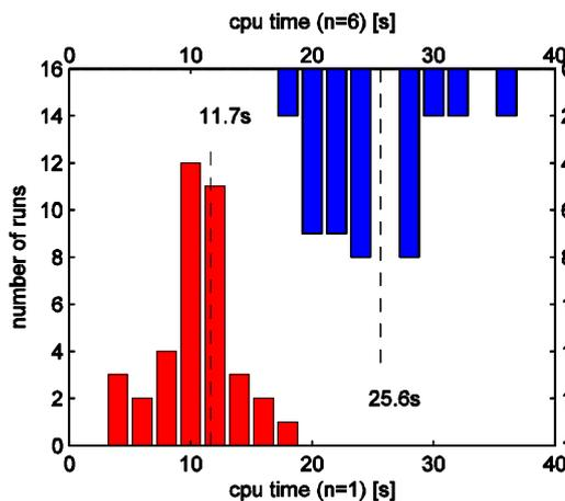
Figure 3 CPU time for multiple MPC executions (SNOPT optimizer), single control structure (red) and optimization of six control structures in parallel (blue)
