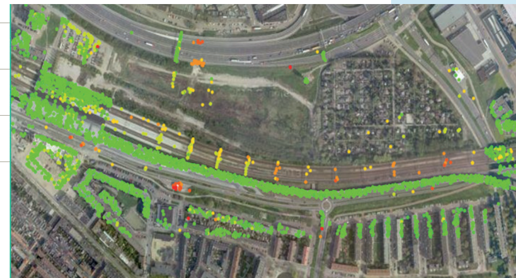
InSAR reflection points on the Hoekse Line (courtesy of SkyGeo)
