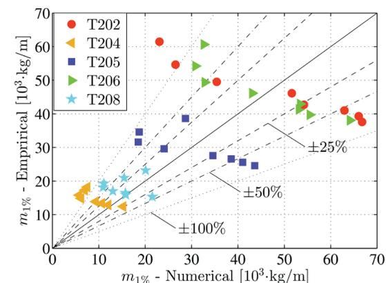
crest wall element was optimised with either an existing empirical formulation from the Rock Manual or with the validated numerical model. This comparison showed that the methods can produce results that can easily vary by a factor of two. More worrying, however, was the fact that the empirical formulations did not necessarily produce conservative results.
