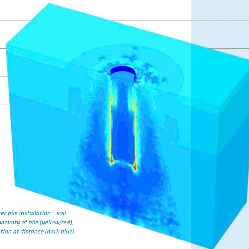
*Void ratio after pile installation – soil loosening in vicinity of pile (yellow/red), soil densification at distance (dark blue)*
