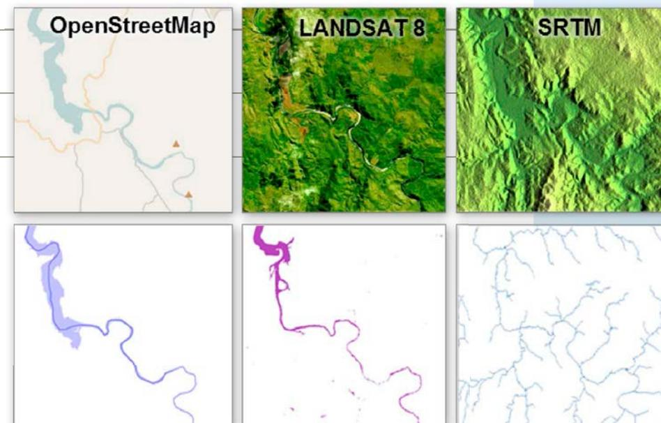
was possible to confirm about 50% of the OpenStreetMap linear water features. The data are clearly complementary. As far as positional accuracy is concerned, the observed differences between river features derived from OSM and Landsat 8 are mostly less than 60 m, which can be considered an excellent match. The differences between the OSM water features and the SRTM analysis are slightly larger (110 m) for the drainage network.
