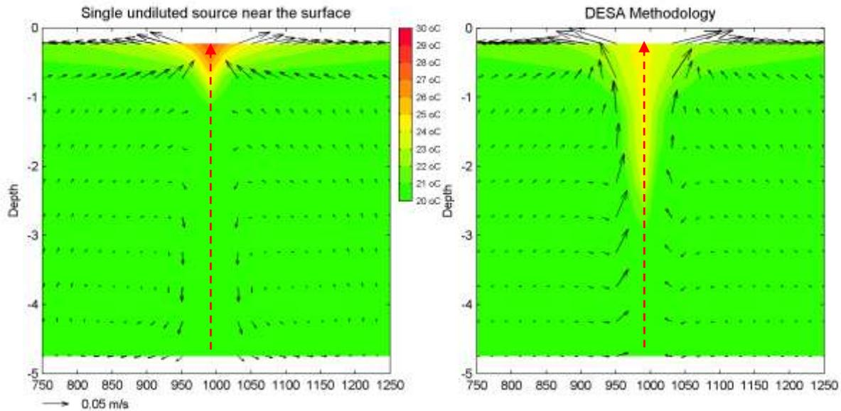
Figure 2 Comparison of flow fields (vertical cross section) in a schematic tank between the traditional, typical method of coupling (left) and the DESA coupling (right). The dashed red arrow shows the jet centreline that is schematised with the two different methods in the model.
