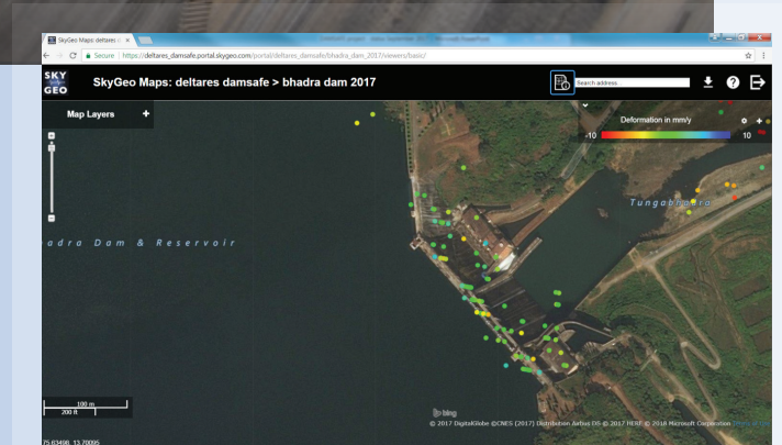
Result of PS-InSAR satellite deformation measurements at the Bhadra masonry dam (courtesy of SkyGeo)
