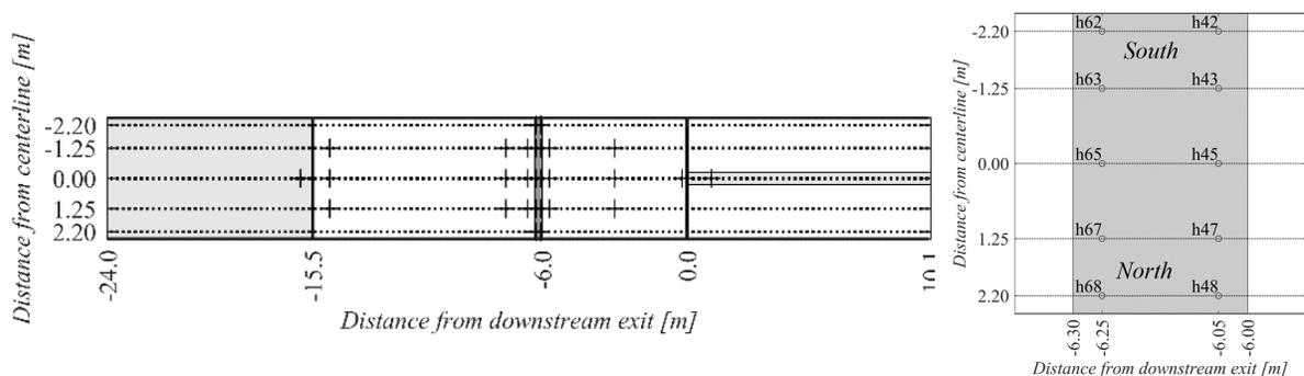
Figure 1. l.h.s.: plan view of the top of the sample, the dark grey area indicates the location of the barrier, the light grey areas indicate the inflow area (from -24 m to -15.5 m) and the outflow area at the ditch (from 0 m to 10.1 m), the white area is covered by the blanket. Crosses indicate locations of PPT's; r.h.s.: close-up of the barrier, transducer row h6# is at the upstream side of the barrier, h4# is on the downstream side of the barrier.
