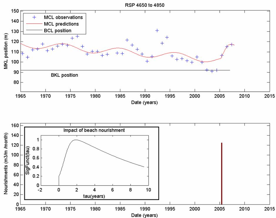
Figure 3.4 (a) Long-term behaviour of the MCL position. Blue dots represent the observations, whereas the solid red line represents the simulated mean trend. (b) Nourishment ( $m^3/m/month$ ) and normalised calculated function representing the impact of beach nourishment on the MCL position
