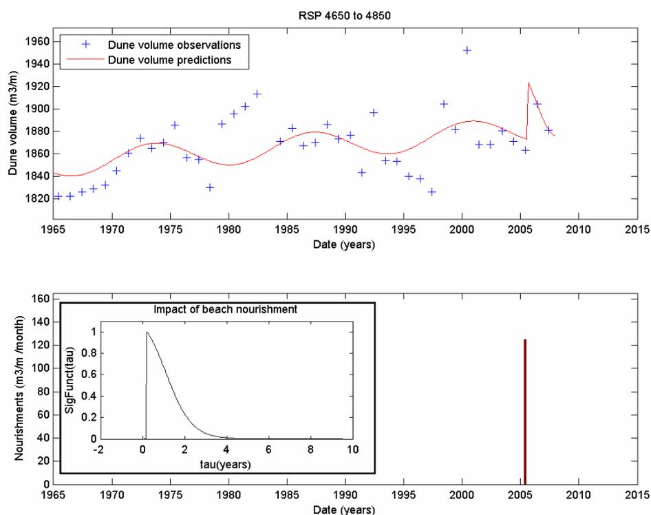
Figure 3.5 (a) Long-term behaviour of the Dune volume. Blue dots represent the observations, whereas the solid red line represents the simulated mean trend. (b) Nourishment ( $m^3/m/month$ ) and normalised calculated function representing the impact of beach nourishment on the dune volume
