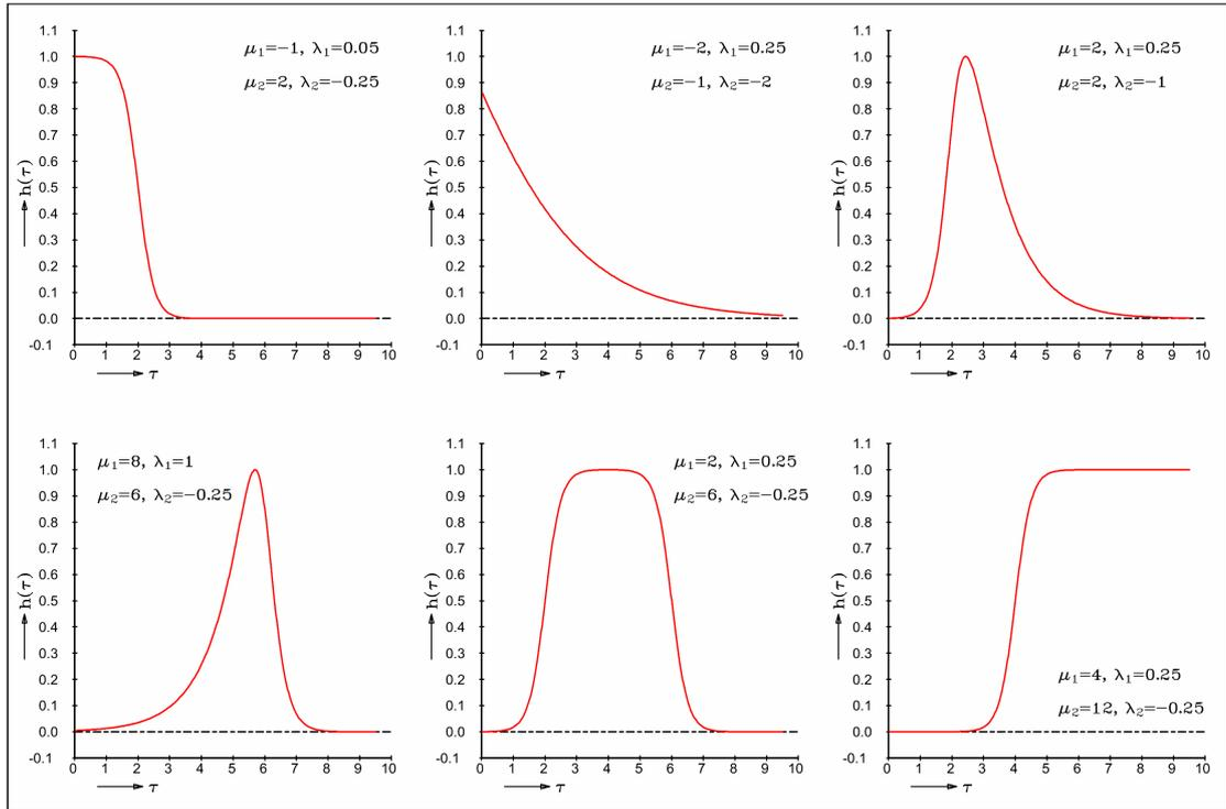
Figure A.1 Plots of parameterised transfer functions  $h(\cdot | \vec{\Theta}_h)$  of Equation A.6 for six variations of the parameter vector  $\vec{\Theta}_h := (\mu_1, \lambda_1; \mu_2, \lambda_2; c)$ . In all case  $c=1$ .
