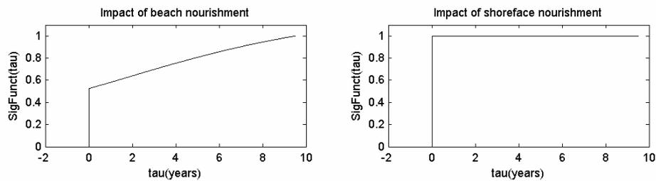
Figure 3.11 Normalised calculated transfer functions representing (a) the impact of a beach nourishment on the MCL position, and (b) the impact of a shoreface nourishment on the MCL position.
