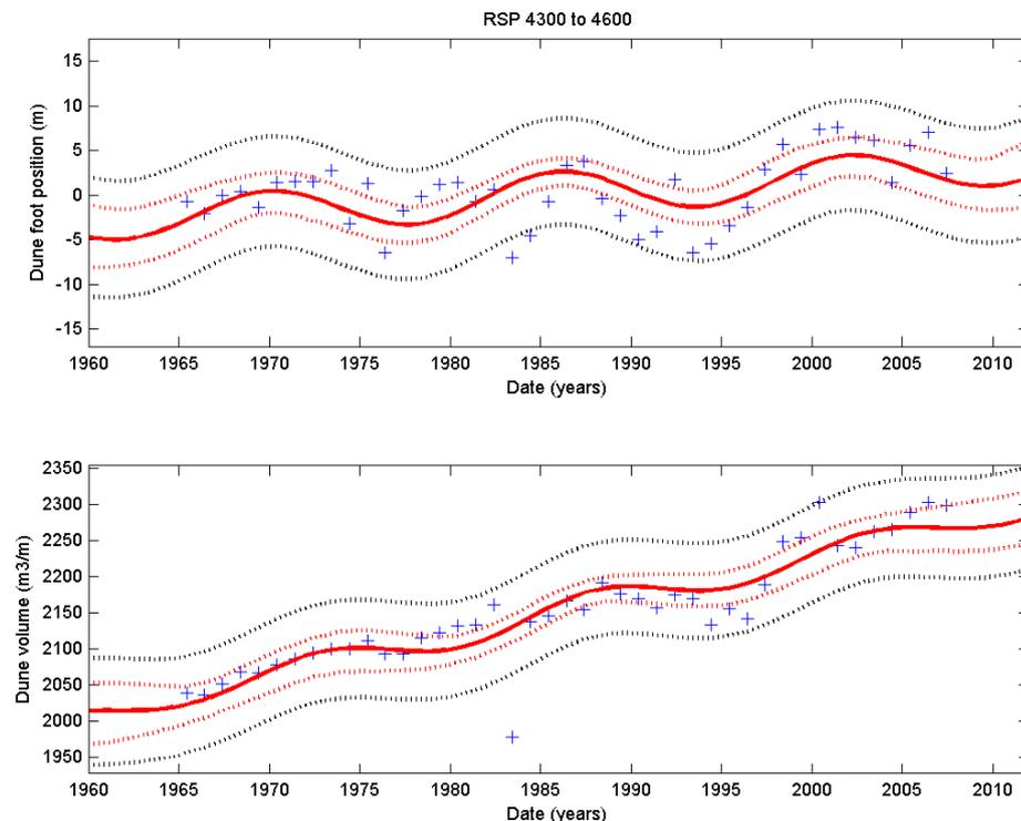
Figure 3.2 Long-term behaviours of CSIs at Egmond-aan-Zee: Dune foot position (m) is displayed on the top panel, where blue dots represent the observations, whereas, the solid red line, the dashed red lines and the dashed black lines represent the simulated mean trend, the boundaries of the 95% skew confidence interval, and the boundaries of the 95% skew prediction interval respectively. The long-term behaviour of the dune volume is displayed on the bottom panel.
