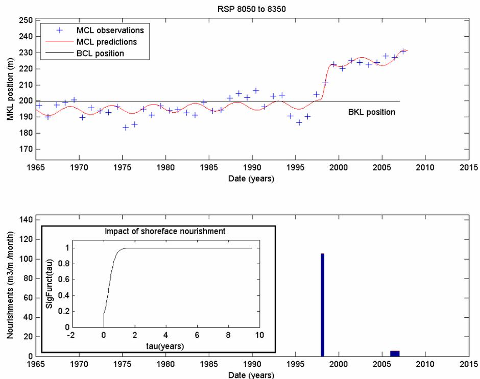
Figure 3.6 (a) Long-term behaviour of the MCL position. Blue dots represent the observations, whereas the solid red line represents the simulated mean trend. (b) Nourishment ( $m^3/m/month$ ) and normalised calculated function representing the impact of shoreface nourishment on the MCL position
