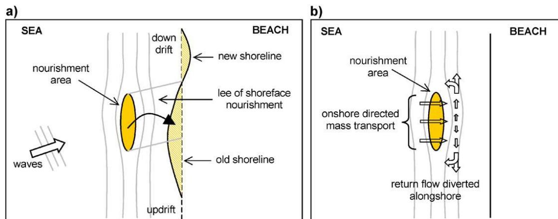
Figure 4.1 Effects expected to occur as a consequence of the placement of a shoreface nourishment (from Duin *et al.*, 2004)
