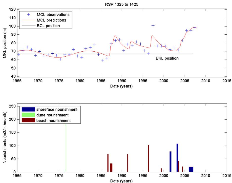
Figure 3.8 (a) Long-term behaviour of the MCL position. Blue dots represent the observations, whereas the solid red line represents the simulated mean trend. (b) Nourishment ( $m^3/m/month$ ).
