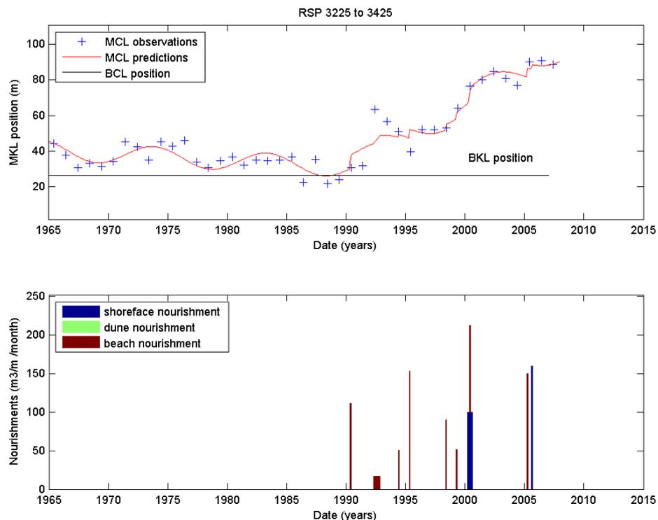
Figure 3.10 (a) Long-term behaviour of the MCL position. Blue dots represent the observations, whereas the solid red line represents the simulated mean trend. (b) Nourishment ( $m^3/m/month$ ).
