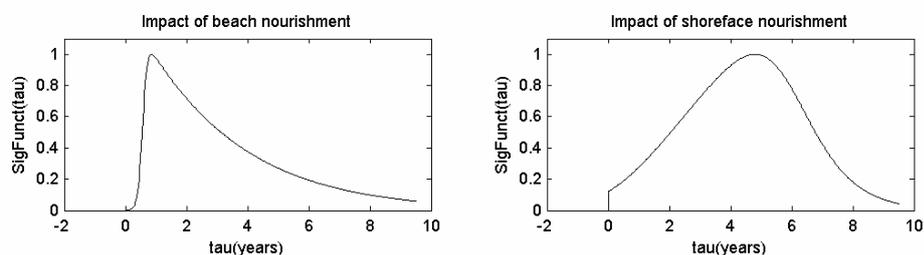
Figure 3.9 Normalised calculated transfer functions representing (a) the impact of a beach nourishment on the MCL position, and (b) the impact of a shoreface nourishment on the MCL position.
