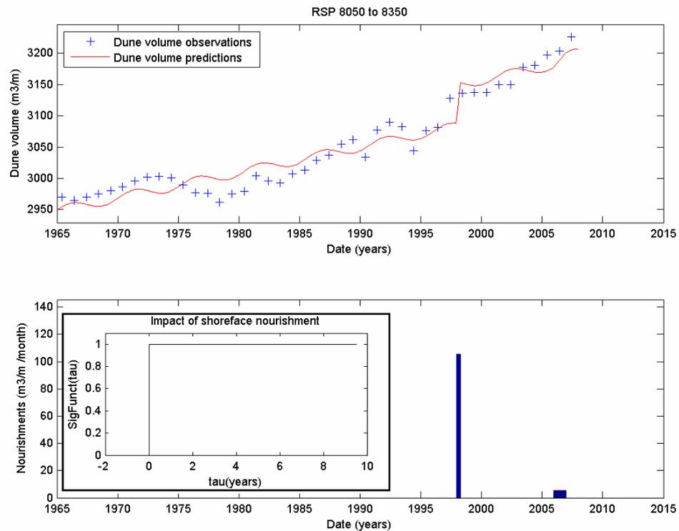
Figure 3.7 (a) Long-term behaviour of the dune volume. Blue dots represent the observations, whereas the solid red line represents the simulated mean trend. (b) Nourishment ( $m^3/m/month$ ) and normalised calculated function representing the impact of shoreface nourishment on the dune volume.
