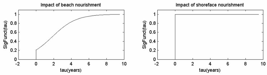
Figure 3.13 Normalised calculated transfer functions representing (a) the impact of a beach nourishment on the dune volume, and (b) the impact of a shoreface nourishment on the dune volume.
