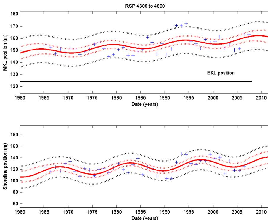
Figure 3.1 Long-term behaviours of CSIs at Egmond-aan-Zee: MCL position (m) is displayed on the top panel, where blue dots represent the observations, whereas, the solid red line, the dashed red lines and the dashed black lines represent the simulated mean trend, the boundaries of the 95% skew confidence interval, and the boundaries of the 95% skew prediction interval respectively. Similarly, long-term behaviour of the shoreline position is displayed on the bottom panel.
