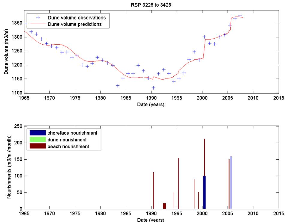
Figure 3.12 (a) Long-term behaviour of the dune volume. Blue dots represent the observations, whereas the solid red line represents the simulated mean trend. (b) Nourishment ( $\text{m}^3/\text{m}/\text{month}$ ).
