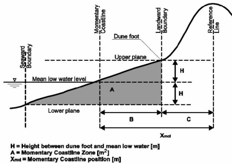
Figure 1.1 Calculation of the Momentary Coastline, MCL; source: Min V&W (1991).
