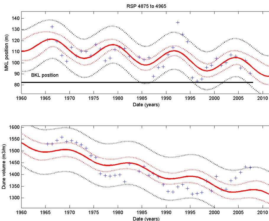
Figure 3.3 Long-term behaviours of CSIs at Egmond-aan-Zee: MCL position (m) is displayed on the top panel, where blue dots represent the observations, whereas, the solid red line, the dashed red lines and the dashed black lines represent the simulated mean trend, the boundaries of the 95% skew confidence interval, and the boundaries of the 95% skew prediction interval respectively. The long-term behaviour of the dune volume is displayed on the bottom panel.
