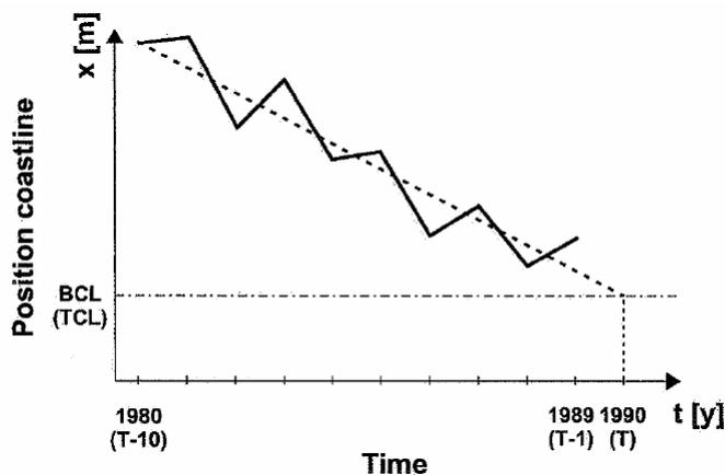
Figure 1.2 Procedure to define the Basal Coastline, BCL, and the Testing Coastline, TCL; source : van Koningsveld and Mulder (2004)
