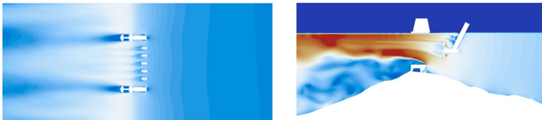
Figure 4.10: Snap-shots of STAR-CCM+ model domain during a simulation with turbines, top- and side-view
