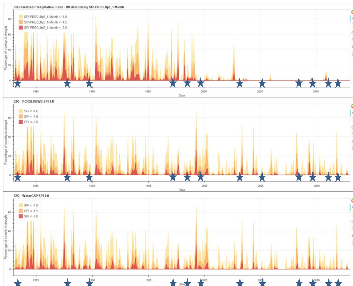
Figure A3.1 – Meteorological drought index SPI1 based on IRI data library (top), based on PCR-GLOBWB (middle), and based on WaterGAP (bottom) for Ethiopia. Grey stars indicate drought events recorded by EM-DAT.
