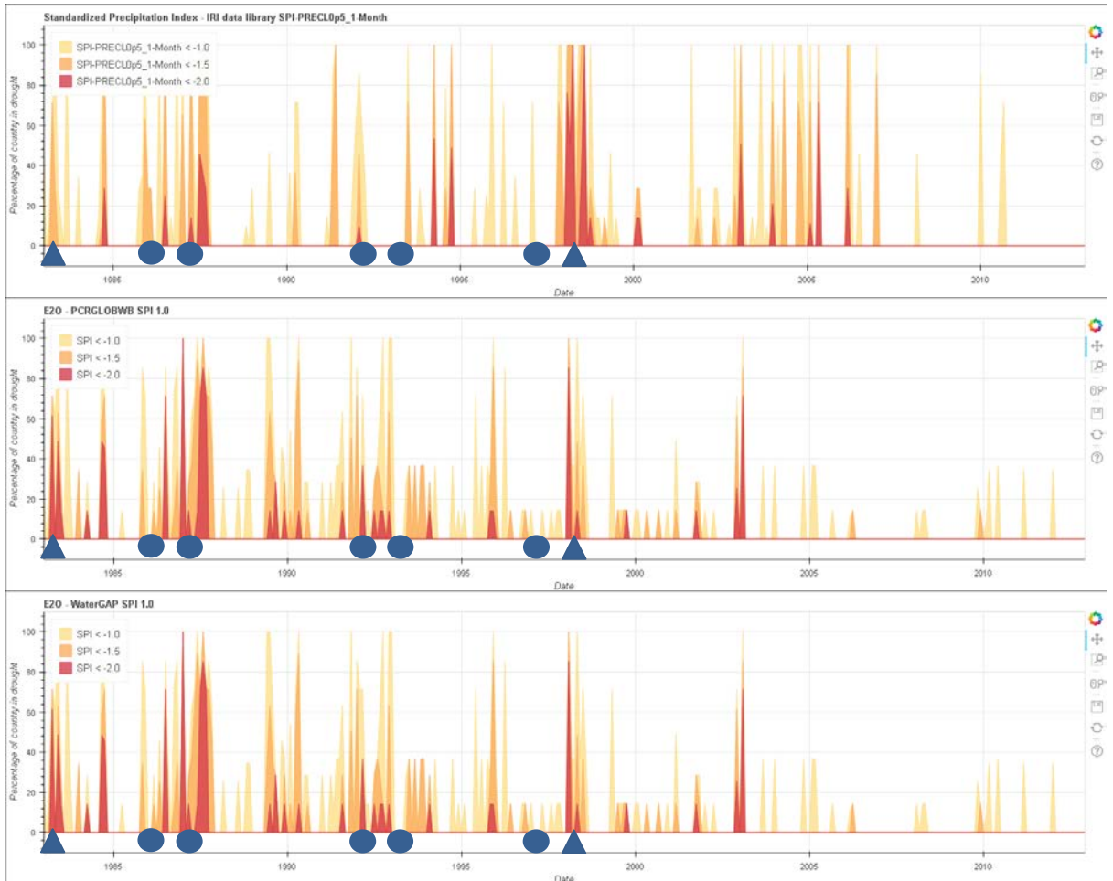
Figure A4.1 – Meteorological drought index SPI1 based on IRI data library (top), based on PCR-GLOBWB (middle), and based on WaterGAP (bottom) for Fiji. Grey dots indicate drought events recorded by Fiji meteorological service; Grey triangles indicate drought events recorded by EM-DAT and Fiji meteorological service.
