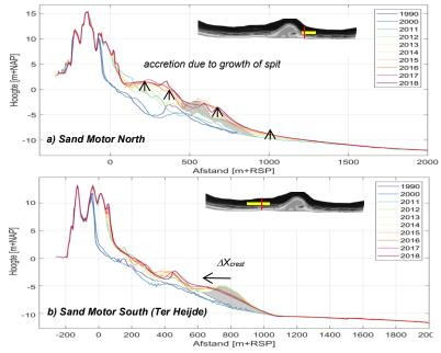
Figure 3.15 Measured cross-shore profiles at the shoreface nourishments close to the Sand Motor. Grey areas demarcate the nourishments (Huisman et al., 2021).
