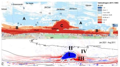
Figure 3.14 Measured bed level change in the period 1993 to 2011 and for the period 2011 to 2018. Accreting areas are shown in red, and erosion in blue.
