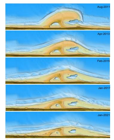
Figure 3.7 Development of the shape of the sub-tidal sand bars for the bathymetries of August 2011 till January 2021 (Huisman et al., 2021).
