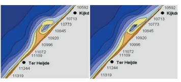
Figure 3.1 The a-priori predicted morphological development of the Sand Motor as computed for the EIA. Left: the computed development after 5 years. Right : the computed morphological change after 10 years.
