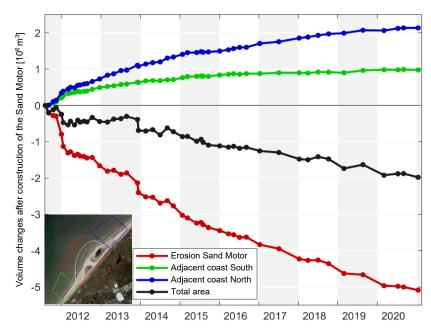
Figure 3.18 Changes in the measured volume of sediment in the first 10 year after construction of the Sand Motor (Huisman et al., 2021).
