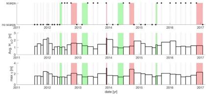
Figure 3.10 Occurrence of cliffs on the Sand Motor in relation to the average wave height ( $H_{s,o}$ ) and wave run-up height ( $\eta$ ). Green : developing cliffs; Red : erosion of cliffs (De Schipper et al., 2017; Van Bemmelen et al., 2020).
