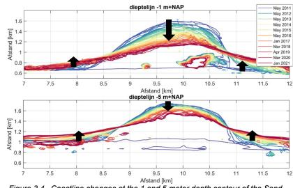
Figure 3.4 Coastline changes at the 1 and 5 meter depth contour of the Sand Motor (Huisman et al., 2021).
