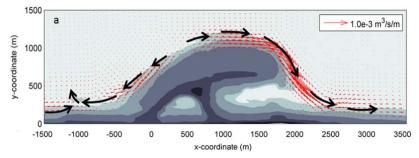
Figure 3.5 Computed year-averaged redistribution of Sand Motor sediment as a result of the obliquely incoming waves (Luijendijk et al., 2017).
