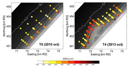
Figure 3.17 Measured median grain size ( $D_{50}$ ) for the situation before and after construction of the Sand Motor.
