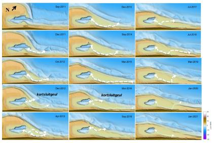
Figure 3.8 Development of the entrance channel at the northern flank of the Sand Motor in the last 10 years. Contour lines show the high-water mark (Huisman et al., 2021).
