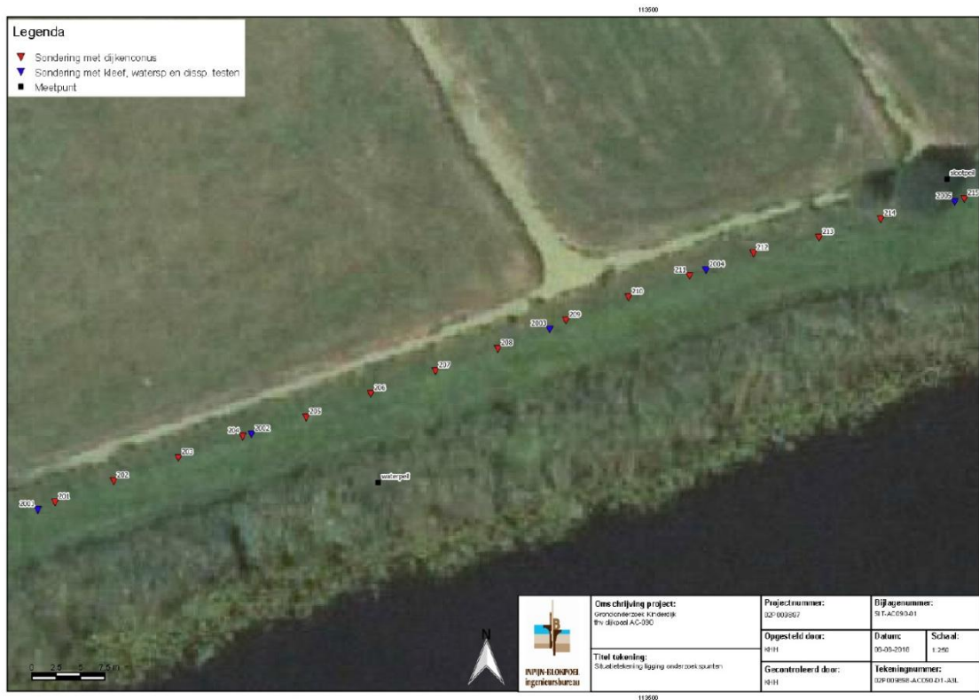
Figure 2.2 Situation of the site AC 090 at the north dike of the drainage canal Achterwaterschap with the locations of the class 1+ cones (red points) and class 1 cones (blue points).
