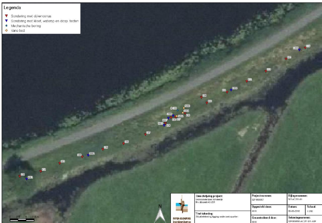
Figure 2.3 Situation of the site AC 251 at the south dike of the drainage canal Achterwaterschap with the locations of the class 1+ cones (red points) and class 1 cones (blue points).
