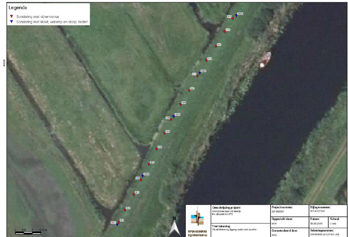
Figure 2.1 Situation of the site AC 075 at the north dike of the drainage canal Achterwaterschap with the locations of the class 1+ cones (red points) and class 1 cones (blue points).
