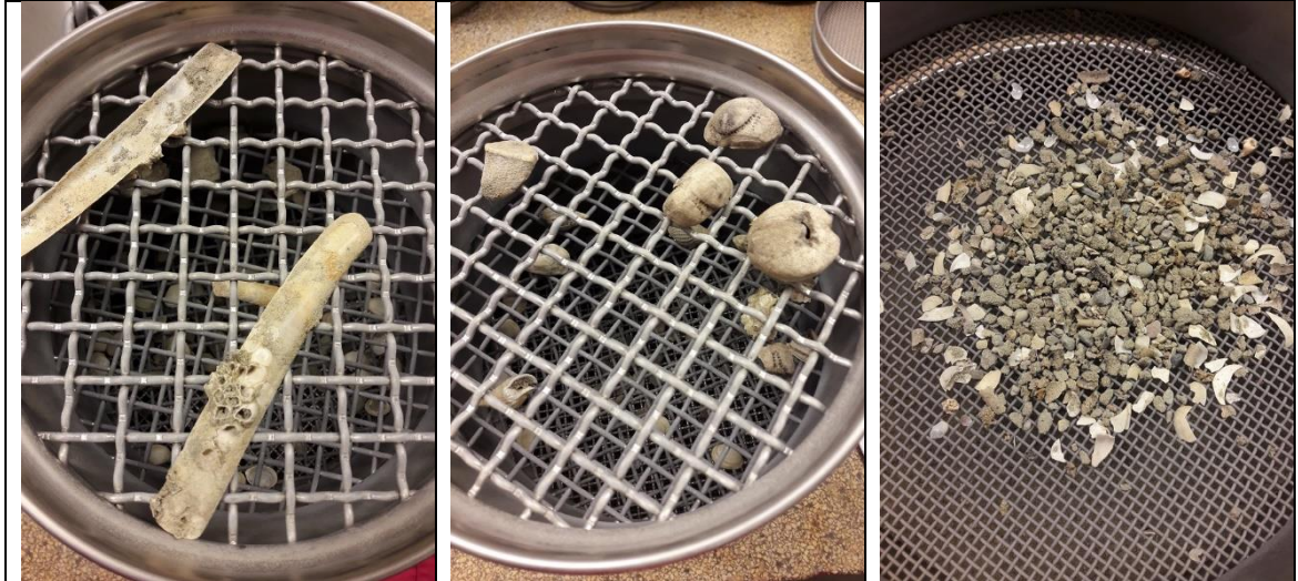
Figure 22: Photos of coarse material on the sieves. Left: BX12, old Ensis sp. on 16-mm mesh and half bivalves on the 8- and 4-mm meshes. Middle: BX16, dead sea urchin crusts on a 16-mm mesh, gastropods on the 10-mm mesh and half bivalves on the 8- and 4-mm meshes. Right: BX16, 2-mm sieve with fine gravel and shell/urchin fragments (carbonate gravel).
