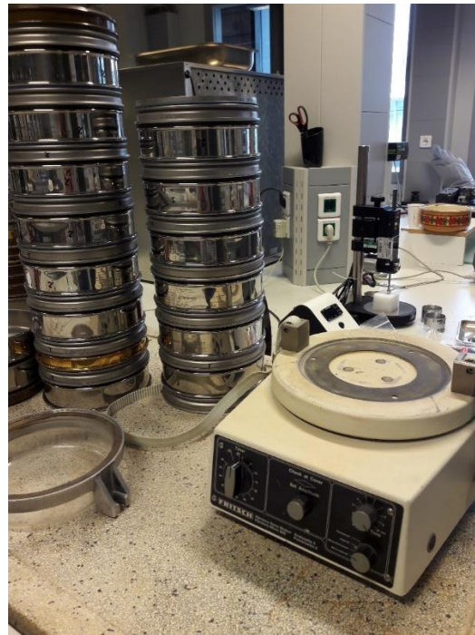
Figure 5: Photo of the sieves and shaking table (on the right), with mesh sizes of stack of sieves used for the larger samples < 2000 \mu\text{m} (in \mu\text{m} ) on the left (according to NEN-5104 standards).
