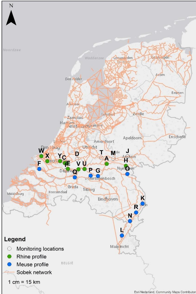
Figure 3.1 Schematization of the Landelijk Sobek model (LSM) version 1.2 and output locations of DELWAQ (circles). Output locations included in the generated river profiles of the Meuse and Rhine are shown in blue and green, respectively. Map was created using ArcGIS 10.6. Labels are assigned to the output locations to increase the readability of the map. The original Sobek IDs and assigned labels are listed in Table 3.1.
