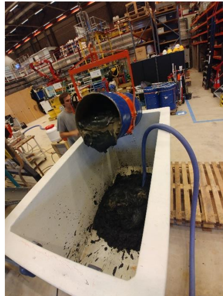
Figure 3-5: Pre-mixing of mud (left-hand side) and deposition of mud into a larger container for dilution.
