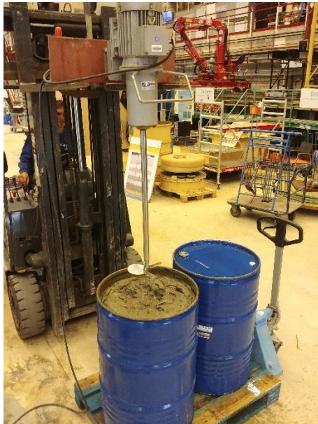
Figure 3-5: Pre-mixing of mud (left-hand side) and deposition of mud into a larger container for dilution.
