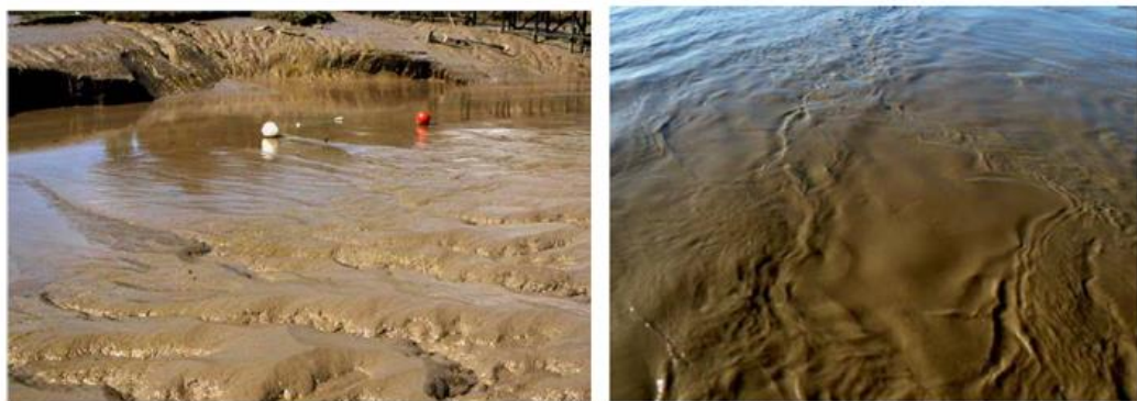
Figure 1-6. Left: stiff consolidated mud. Right: weak fluid mud.
