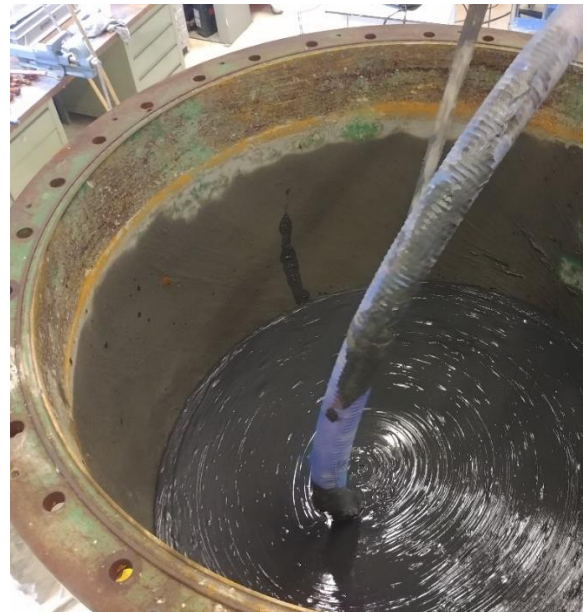
Figure 3-6: Mixing of the mud in the large collection container (left-hand side) and filling of the test container (right-hand side).
