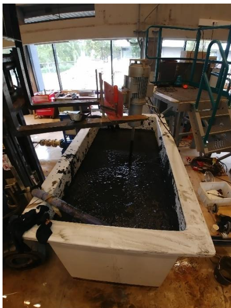
Figure 3-6: Mixing of the mud in the large collection container (left-hand side) and filling of the test container (right-hand side).
