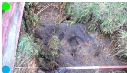
Figure 1.3.4. Ol.3 N = 1000 detail damage
