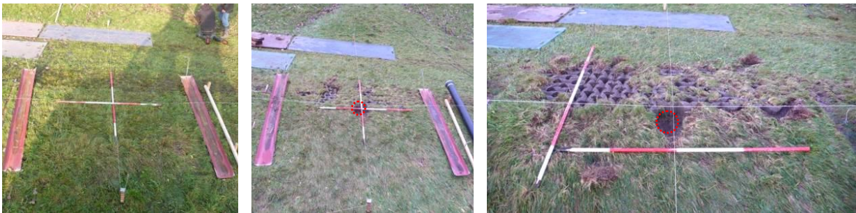
Figure 8. Impression of damage development and artificial damage of Test Section Be.2. Artificial damage is indicated with red circle. Left: initial condition, middle: after 1500 impacts, right: after 3500 impacts.
