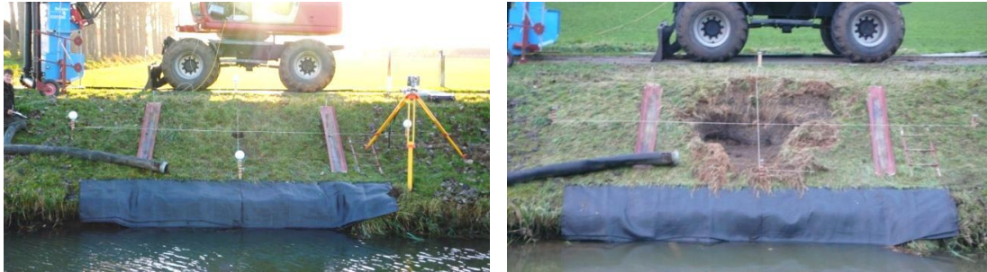
Figure 15. Left: initial condition at Ol.1. Right: after 3000 impacts.
