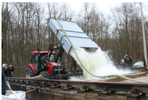
Figure 24. Impression of alternative wave impact generator that can generate impacts with a larger load.
