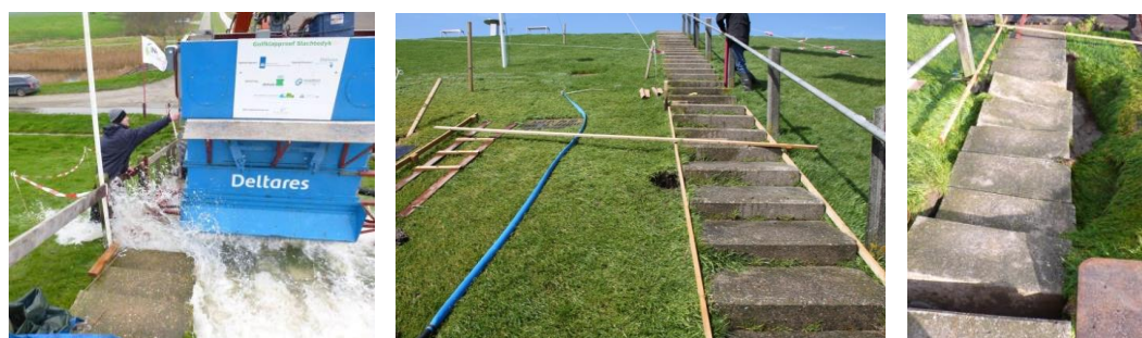
Figure 3. From left to right: impression of testing at the stairs, initial condition (Oo.4), condition after 1000 impacts (Oo.4).
