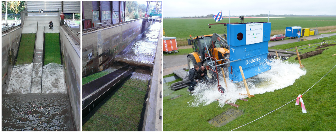
Figure 1. Impression of testing grass dikes in the Deltares Delta Flume (left and middle) and with use of the wave impact generator (right).
