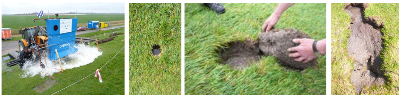
Figure 2. Impression of testing at reference section (Oo.1). From left to right: impression during testing, initial situation, after 860 impacts, after 7001 impacts.
