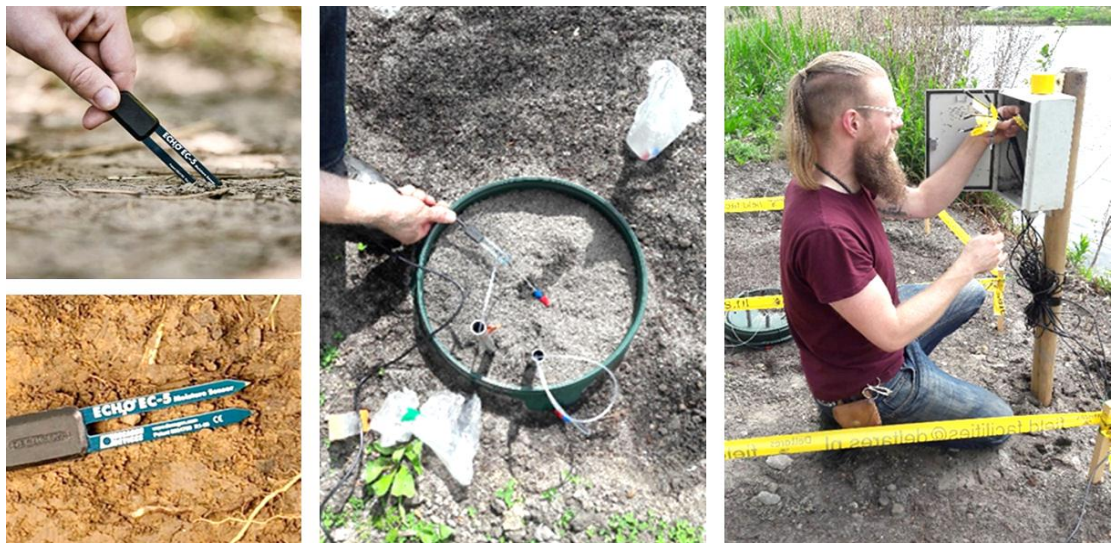
Fig. 3. Moisture sensors, installation and on-site monitoring via dataloggers.
