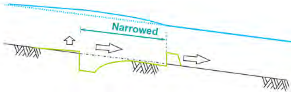
Figure 1 Short-term effect of narrowing the main channel.
