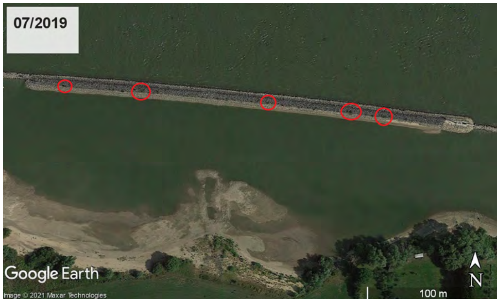
Figure 66 Satellite image of the upstream end of the longitudinal training wall at Wamel in 2019. Red circles indicate some of the vegetation growing.
