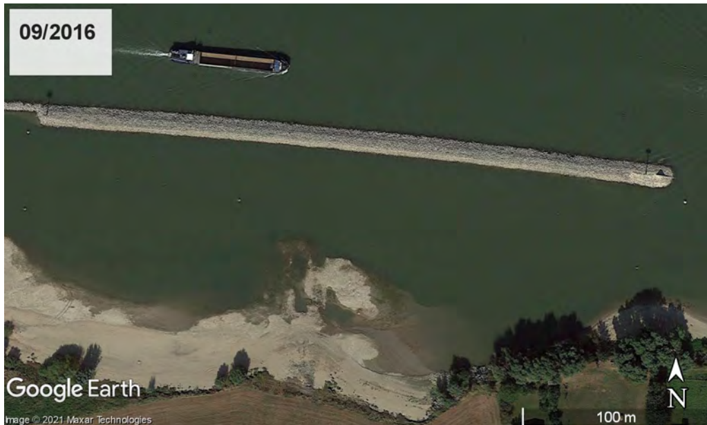
Figure 64 Satellite image of the upstream end of the longitudinal training wall at Wamel in 2016.
