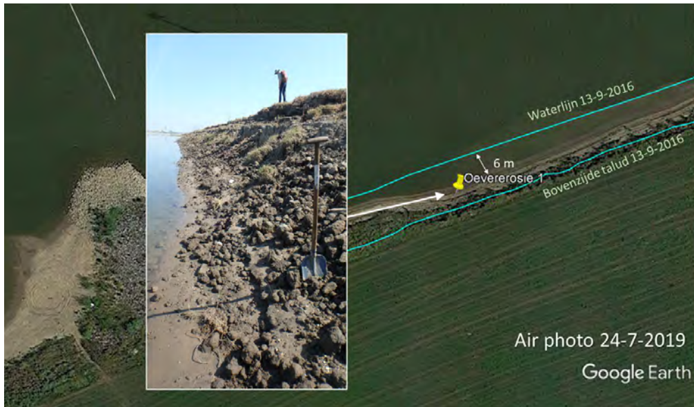
Figure 24 Google Earth® aerial photograph of auxiliary channel at Wamel at RKM 913.9 with photograph of the eroding bank at this section (photo taken at location of pin in upstream direction).
