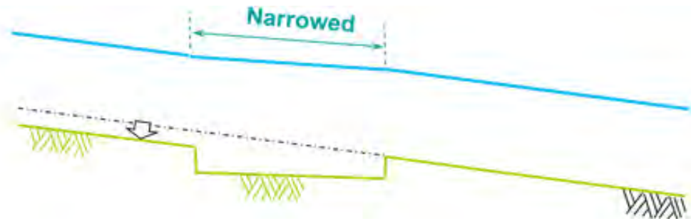
Figure 2 Long-term effect of narrowing the main channel.
