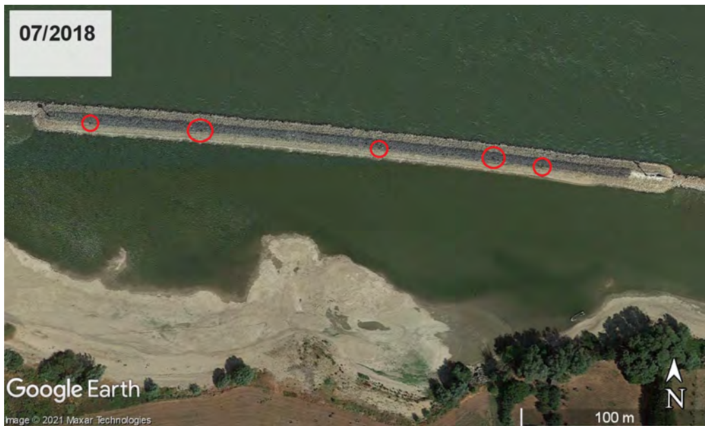
Figure 65 Satellite image of the upstream end of the longitudinal training wall at Wamel in 2018. Red circles indicate some of the vegetation growing.
