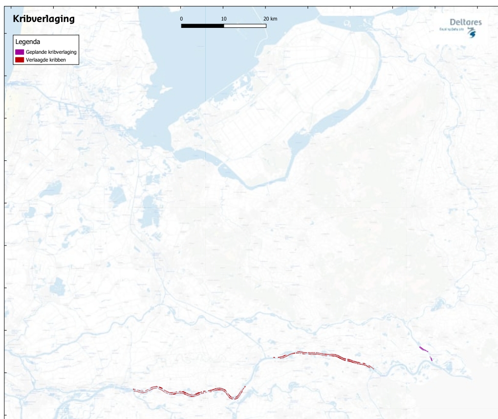
Figure A.13 Groynes that were lowered on the Waal in the program Ruimte voor de Rivier. Source: Buijse et al. (2019)
