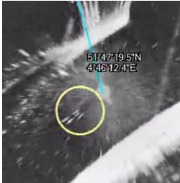
Figure 3-11: Radar image of the plastic items at 12:54 on 6th March 2020. 5 distinct signals could be observed approximately 100m from the radar. Using visual corroboration, the plastic signal was marked out manually (yellow circle). The coordinates in the image belong to the center of the yellow circle, in this case, the location of the plastic items.
