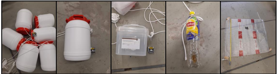
Figure 2-3: Types of plastic items attached to the rope that was deployed on 4 March 2020. To ensure sufficient buoyancy of some of the materials, makeshift buoys were attached to them made of low-density wood. All items used in these measurement campaigns were successfully retrieved.
