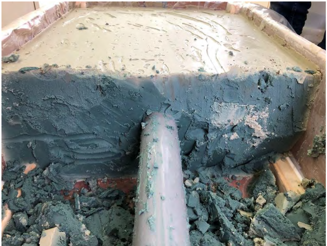
Figure 3.1 Test on frictional behavior drill grout
