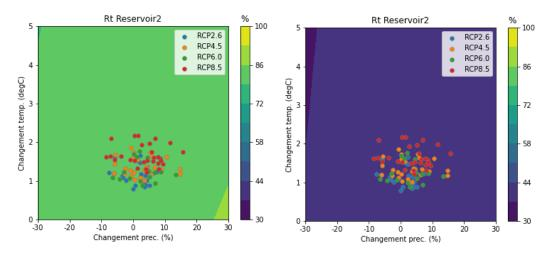
The graphs above provide the same information but now for the situation where a large reservoir upstream of Ntoum is build within the river system. The change to slightly lighter colors indicates that the reservoir will improve water availability a bit. The request can be satisfied for an additional 5% of time. Here only the results for this
