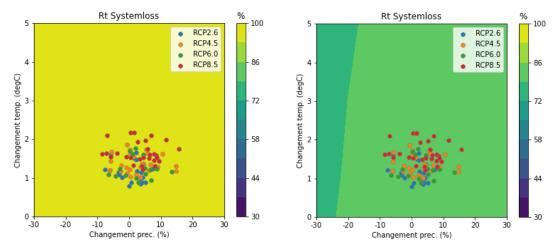
The largest improvement can be achieved by decreasing the losses of the distribution system from the Ntoum treatment plant to the city of Libreville and its inhabitants. In the improved situation where the efficiency of the distribution network is increased from 52% to 71%, the demand can be satisfied (100% of time) by only considering future climate change (left). When the future increasing demand is also considered, demand can be satisfied for at least 82% of the time (right).
