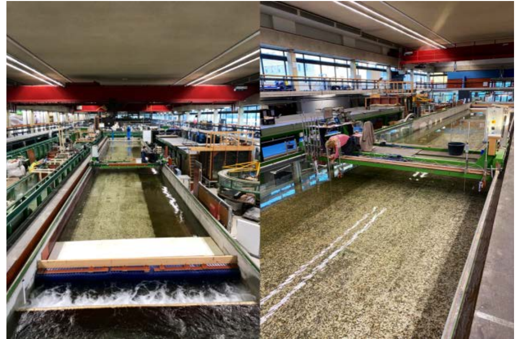
Overview of the Laboratory test setup (before installing groynes)
