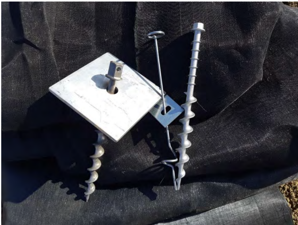
Figure 2.2 Spiral pins (screw peg) with plate (washer) for a better fixing of the fabric (from left to right: Wurmi, Gripple, Peggy Peg). These pins have to be placed by using an adapter and a cordless screwdriver
