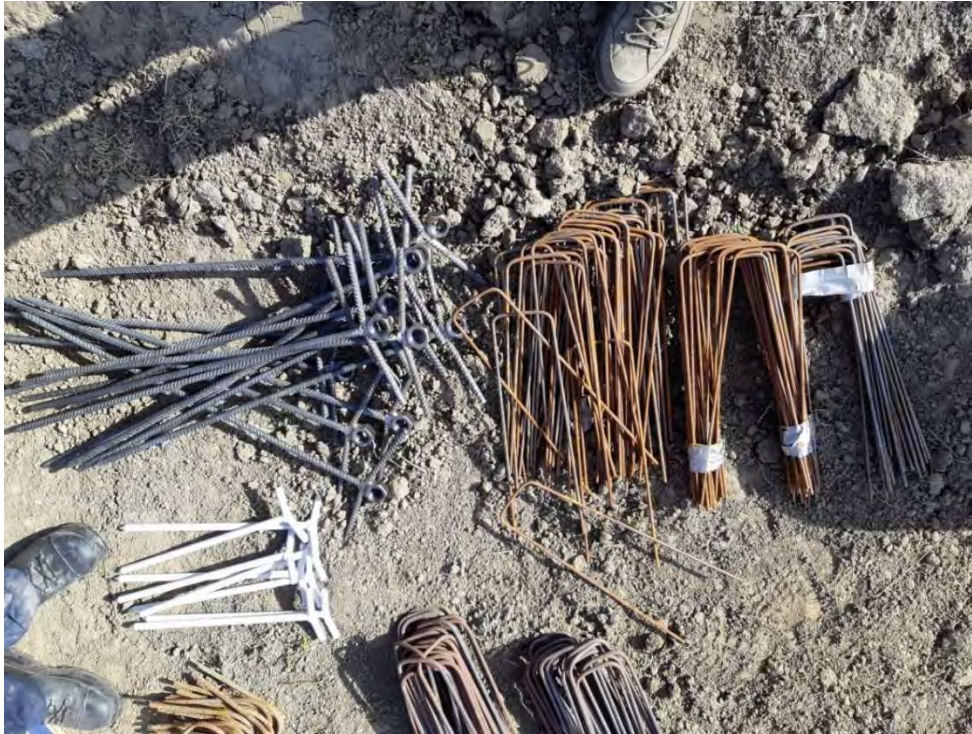
Figure 2.1 Different types of pins for fixing the panels on the ground (amongst others: U-, Y -form)
