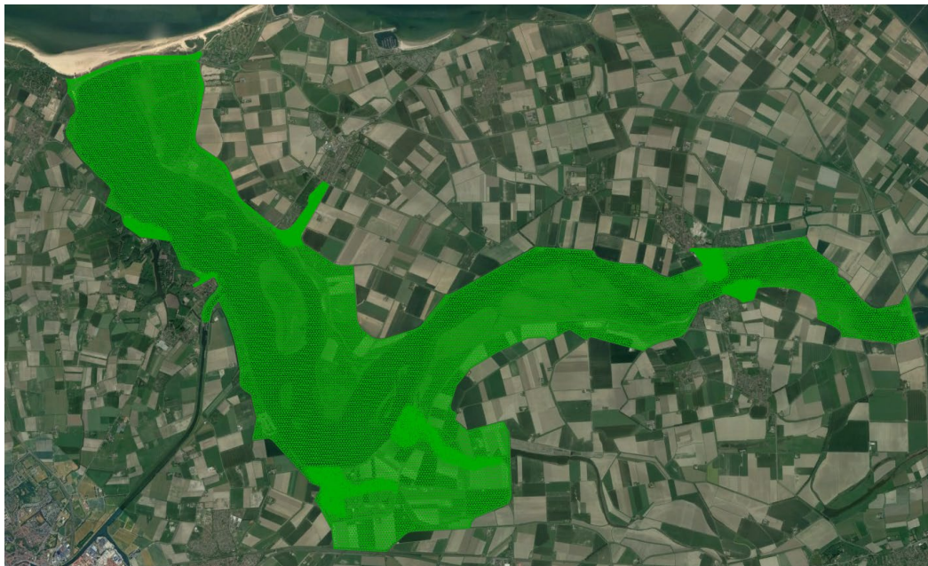
Figure 3.1 Computational model domain of online-coupled D-HYDRO and D-Water Quality model for Veerse Meer
