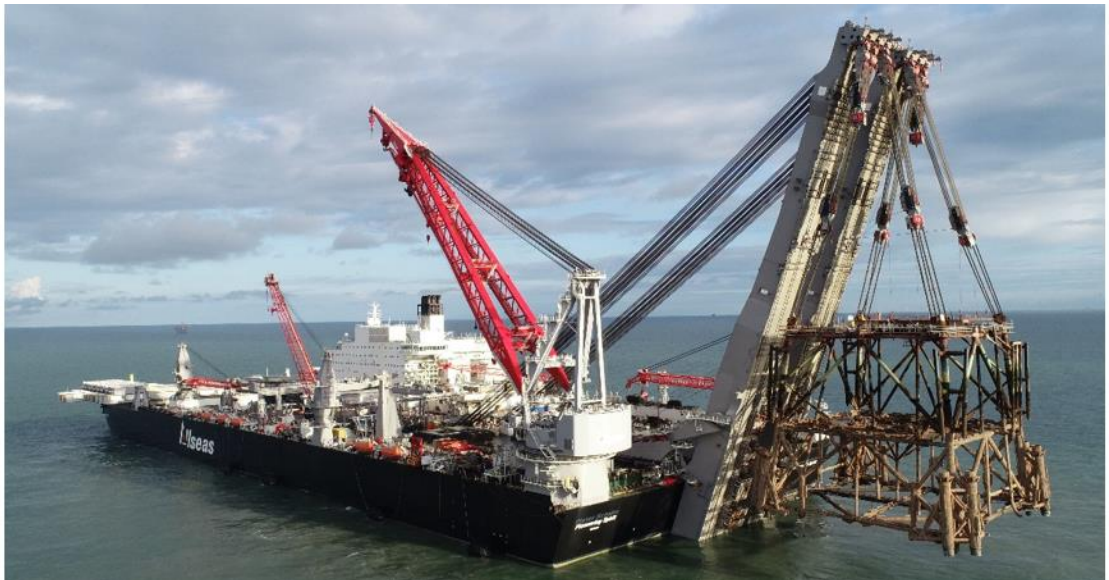
Figure 6.4 Allseas Morecambe project. The Pioneering Spirit lifting the first offshore jacket. Operations are timed favourably (during slack water) by means of the TKI Ocean Race Pilot.
