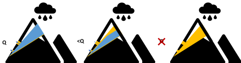
Figure 2-5 Schematic showing how a landslide can (temporarily) block the recharge zone (right side of the mountain, indicated by the black continuous line) and how this could lead to reduced spring discharge or drying up of the springs by reducing the groundwater table. In the figure, the black colour indicates the impermeable bedrock, the yellow colour the porous parts / aquifer and the blue colour indicates the water table.
