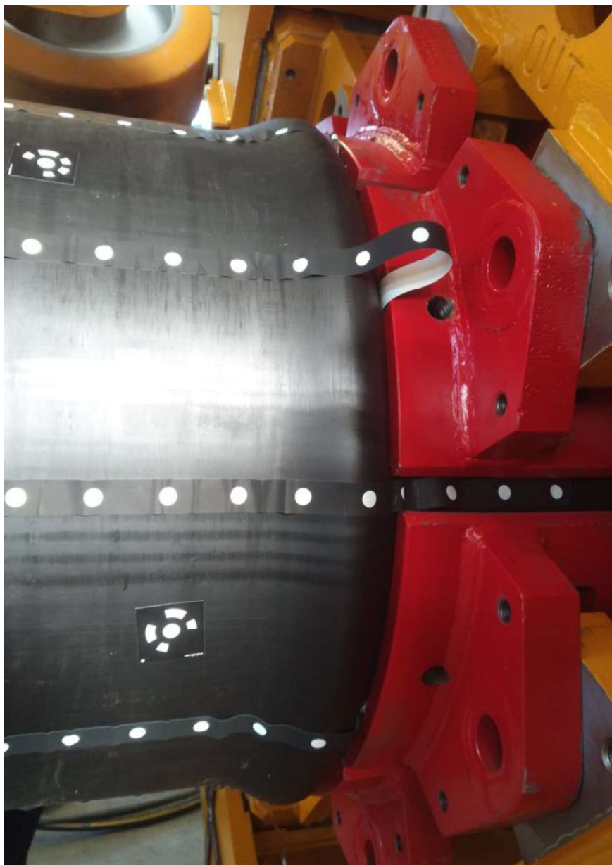
Figure 92: Compressed HDPE pipe at 50 bar clamping and 60 bar thrust
