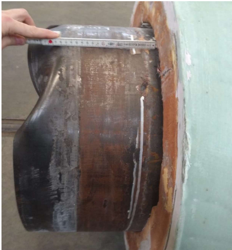
Figure 171: Movement of HDPE PUR GRP
