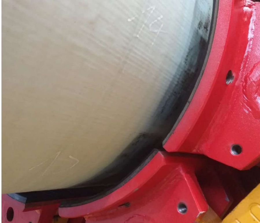
Figure 63: No damage visible after 275 bar clamping pressure
