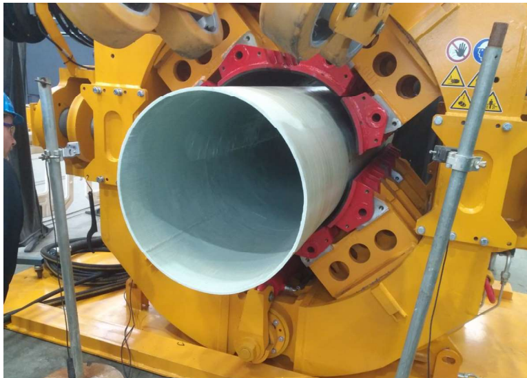
Figure 8: Placed GRP pipe in the clamping unit
