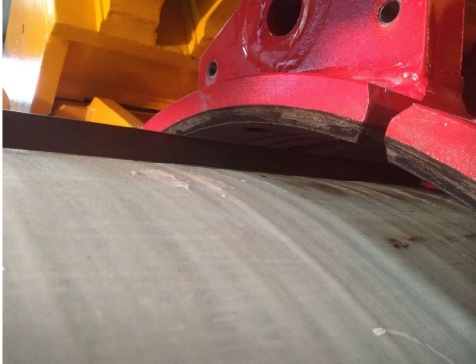
Figure 51: No damage visible after 110 bar clamping pressure
