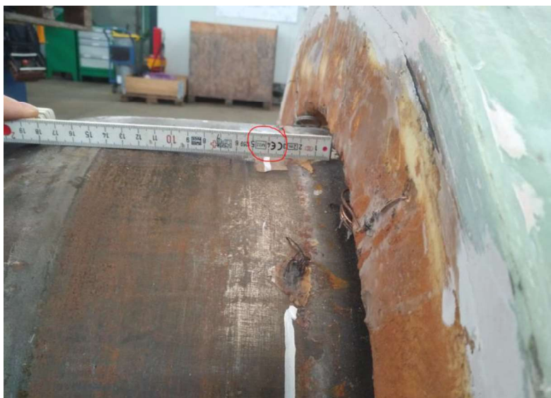
Figure 172: Movement of HDPE PUR GRP
