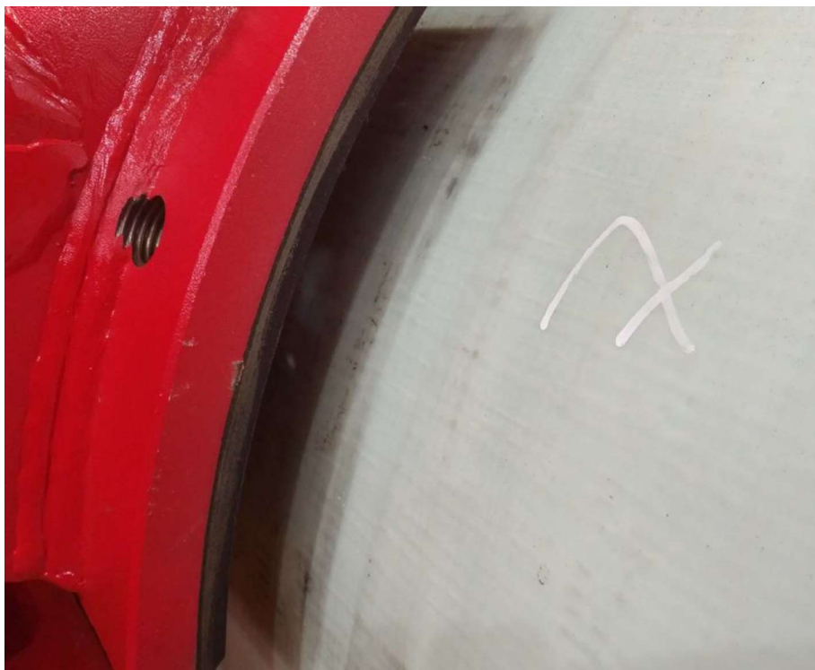
Figure 61: Figure 56: No damage visible after 275 bar clamping pressure
