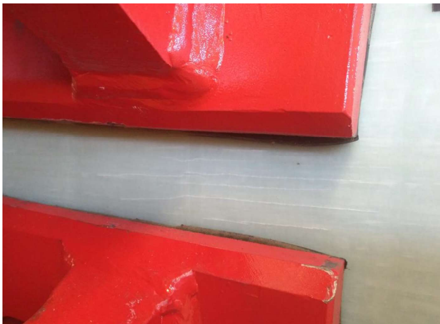
Figure 131: Damage between the side clamps
