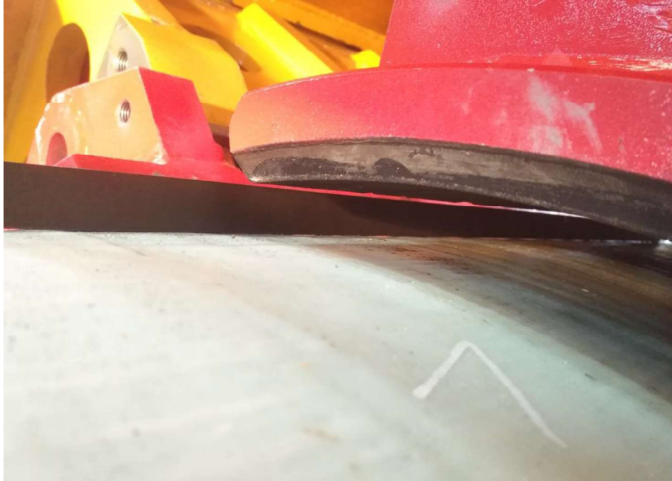
Figure 59: No damage visible after 275 bar clamping pressure
