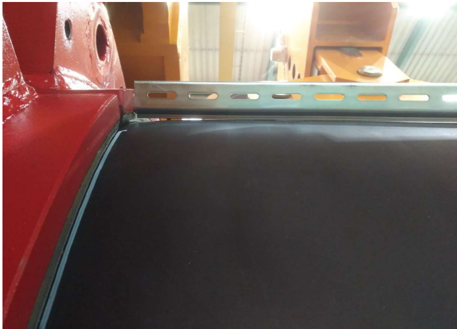
Figure 89: Elastic deformation of the pipe at 50 bar clamping and 0 bar thrust
