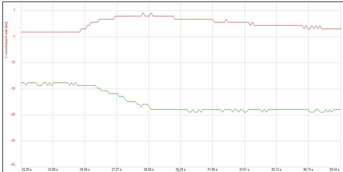
Figure 102: Pressure of clamps and movement of clamping unit as a function of time (second test)
