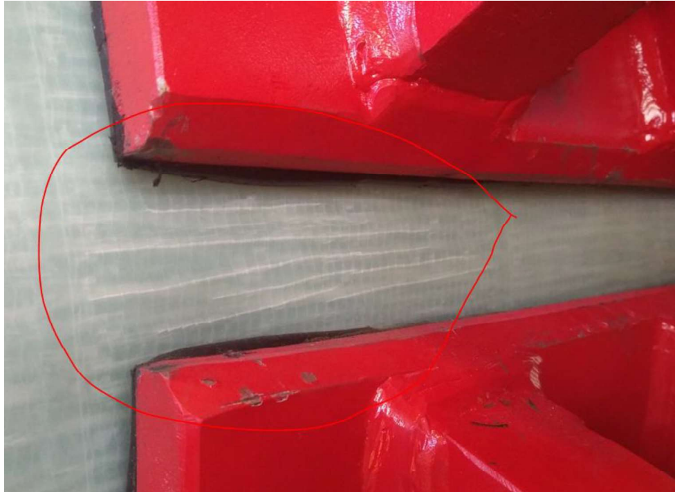
Figure 128: Damage of the pipe between the side clamps
