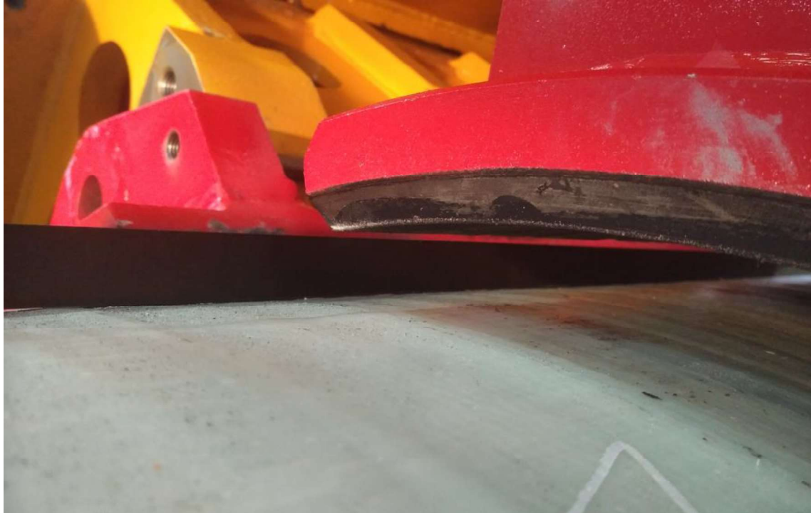
Figure 53: No damage visible after 170 bar clamping pressure
