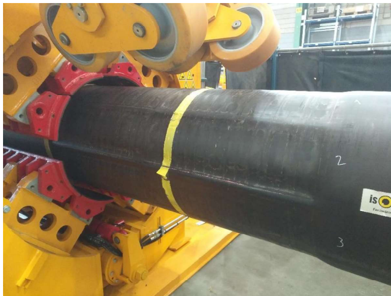
Figure 34: HDPE pipe before clamping
