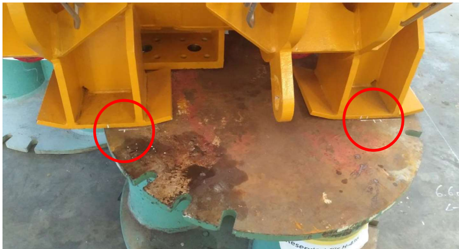
Figure 98: Displacement of the clamping unit
