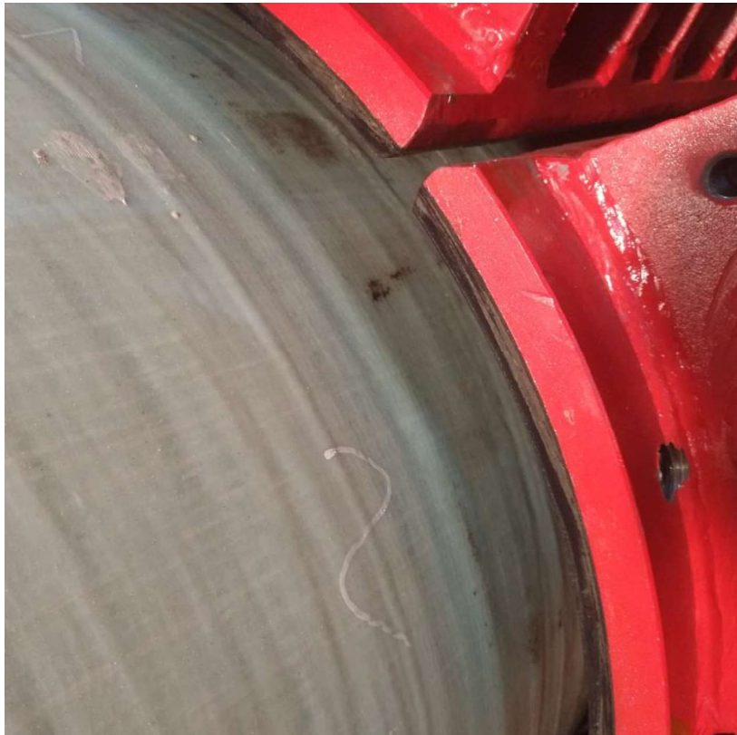
Figure 50: No damage visible after 86 bar clamping pressure
