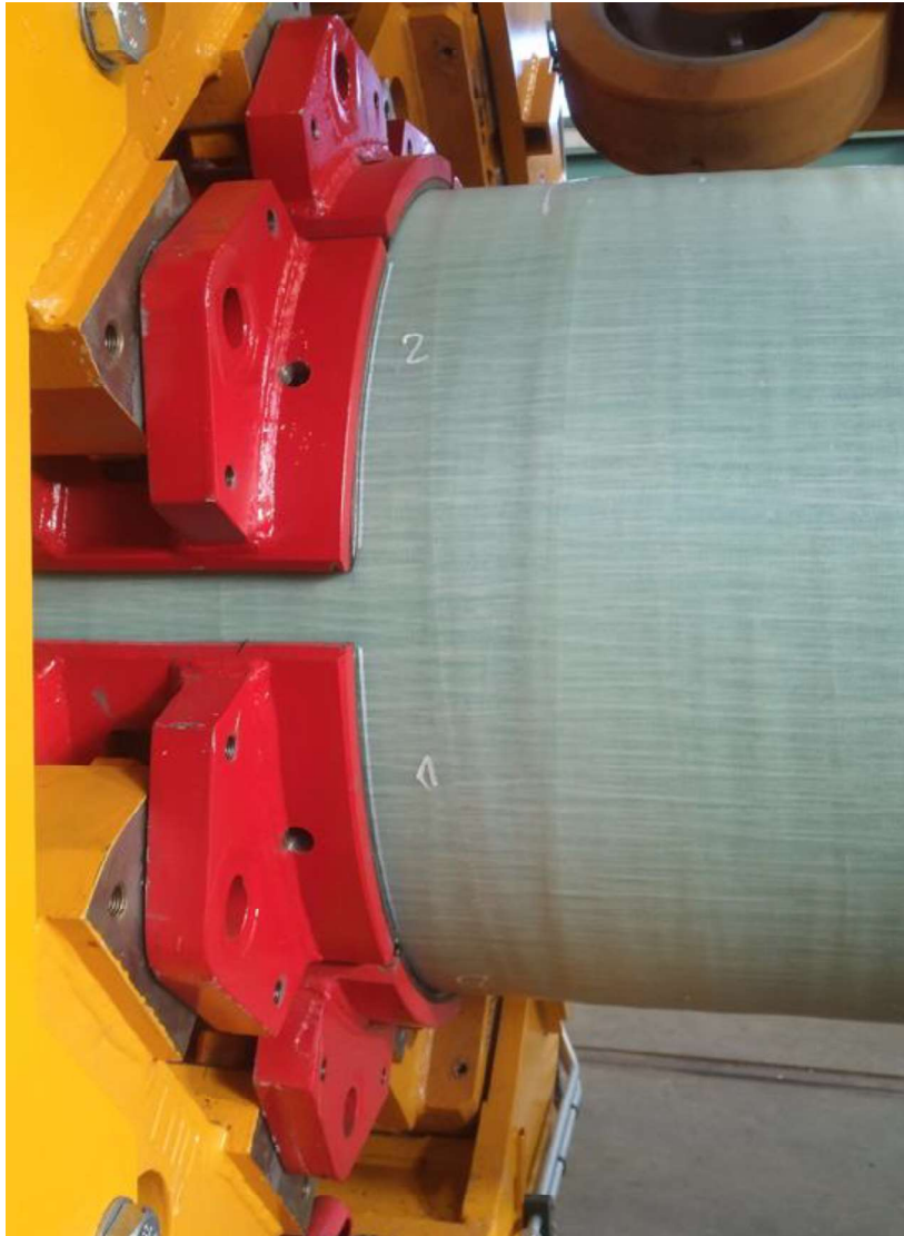
Figure 108: Marks for detecting slip
