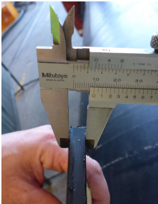
Figure 96: Wall thickness of nearly 10 mm in the non-stressed area
