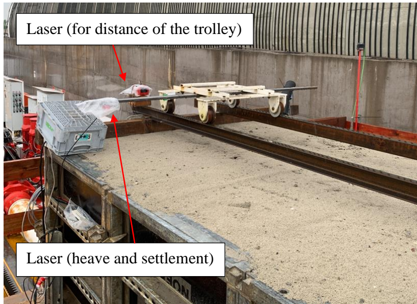
Figure 16: Trolley for detection of heave and settlement
