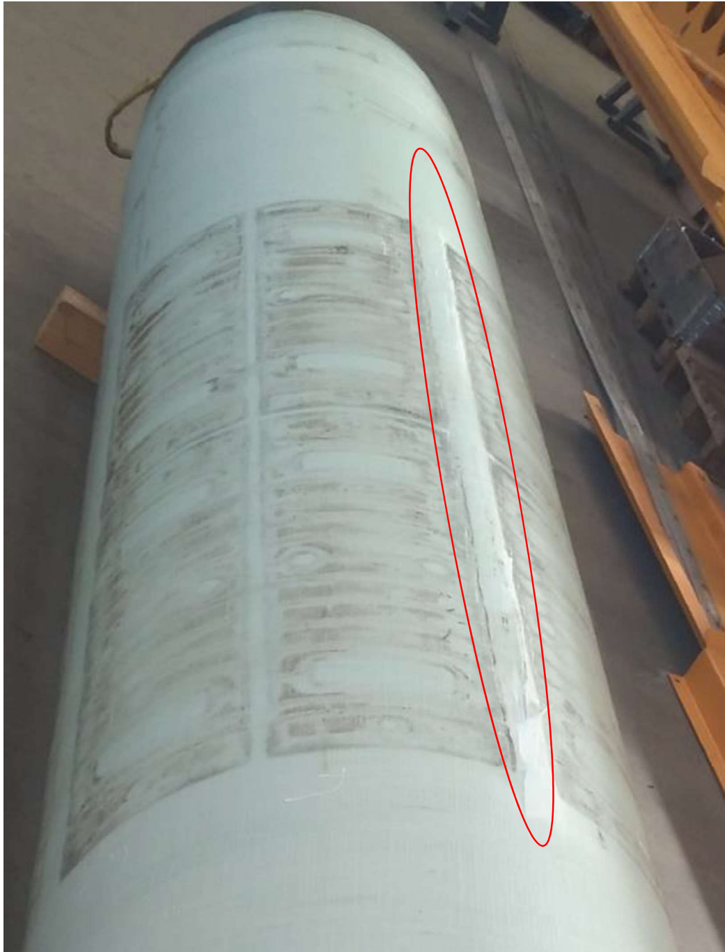
Figure 71: Damaged pipe after disassembly
