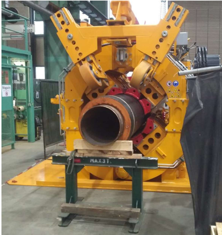
Figure 25: 16 m HDPE pipe placed in clamping unit
