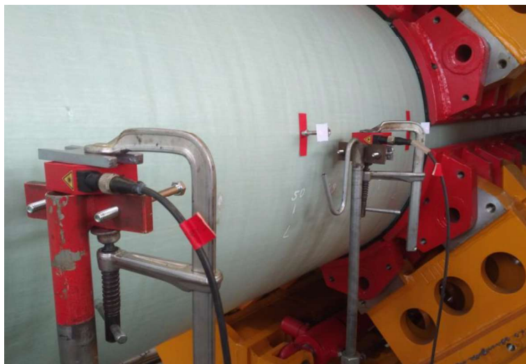
Figure 143: Two lasers for measuring axial deformation
