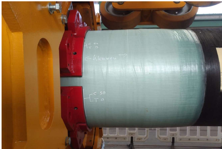
Figure 145: Marks to detect slipp
