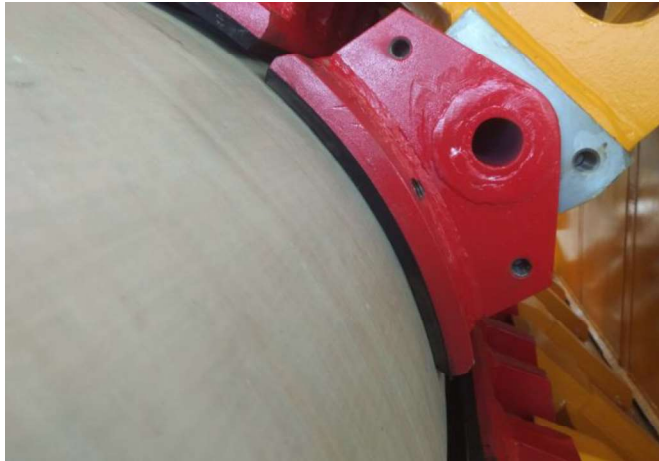
Figure 10: Contact between clamps and pipe
