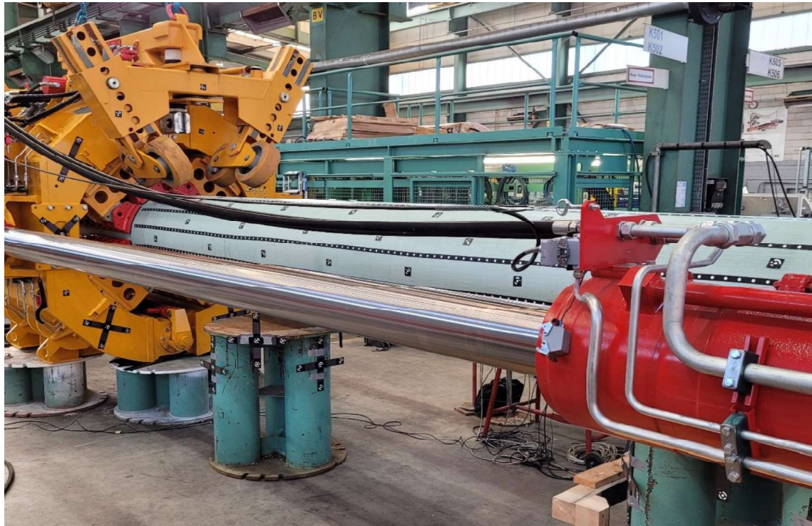
Figure 105: Axial test setup with 16 m HDPE GRP pipe
