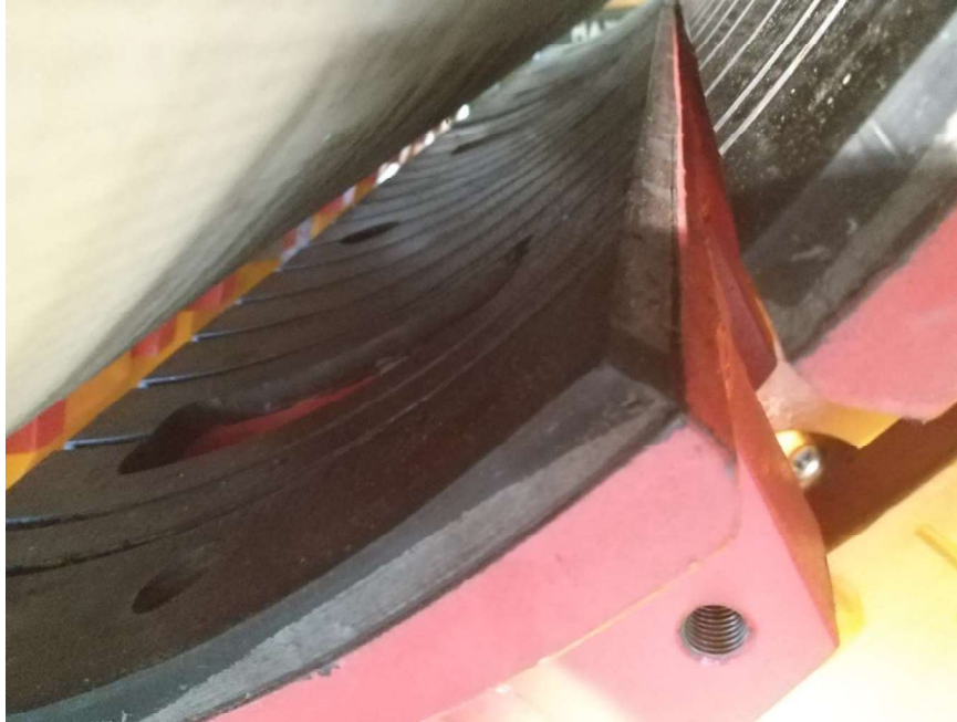
Figure 72: Condition of clamps after test
