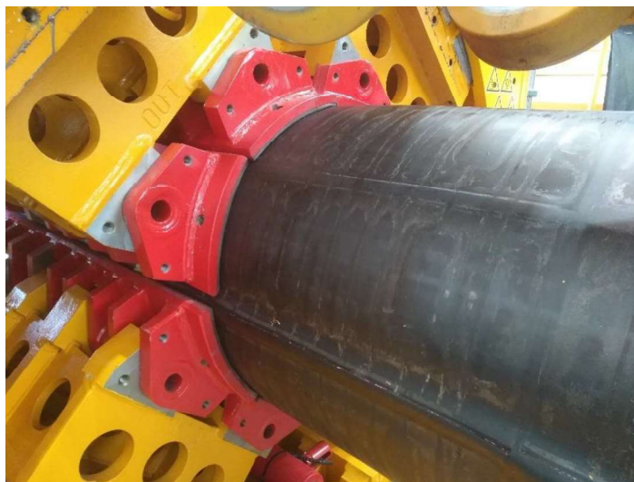
Figure 36: Clamped pipe at second test
