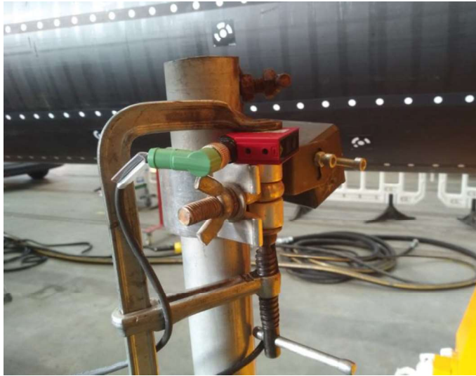
Figure 77: Laser between fixed ground and clamping unit
