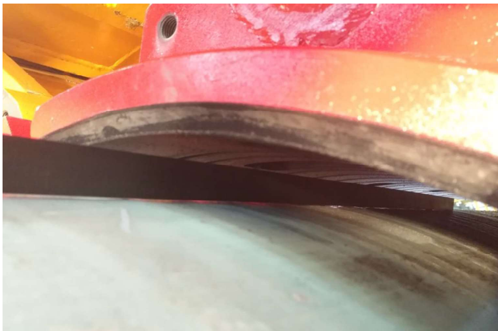
Figure 55: No damage visible after 240 bar clamping pressure
