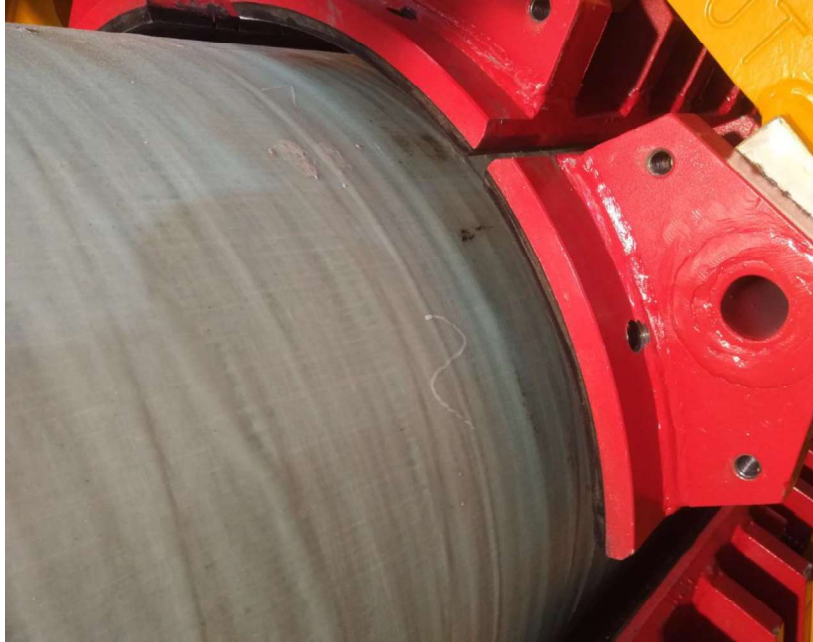
Figure 49: No damage visible after 60 bar clamping pressure
