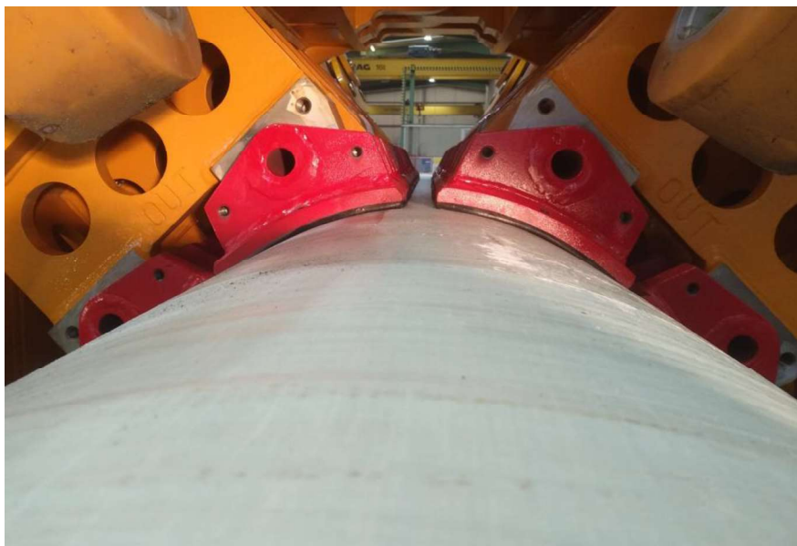
Figure 58: Clamping with full 275 bar (no damage recognised)
