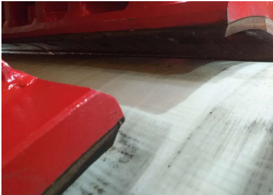
Figure 60: Figure 56: No damage visible after 275 bar clamping pressure
