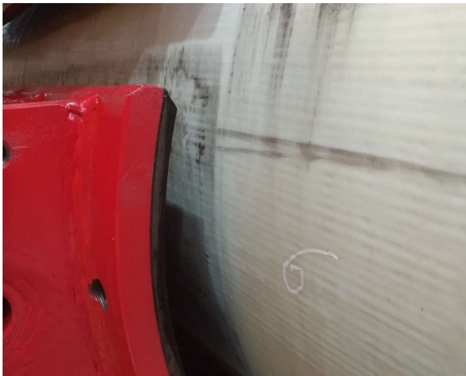
Figure 62: No damage visible after 275 bar clamping pressure
