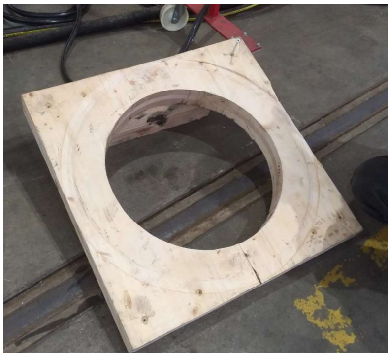
Figure 167: Compressed wooden plate
