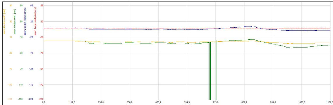
Figure 151: Graph of movement of thrust unit (red), clamping unit (blue), reflector 1 (green) and reflector 2 (yellow) as a function of time
