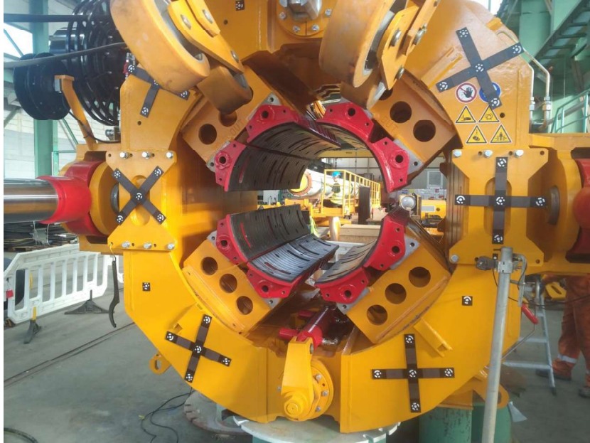
Figure 75: Measuring points at the clamping unit
