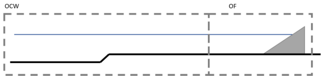
Figure A.2 Model set-up of the numerical simulations based on the Scheldt Flume 2018 experiments (Deltares, 2019). The model is composed of an OceanWave3D domain (left) and OpenFOAM domain (right) to reduce the computation time.
