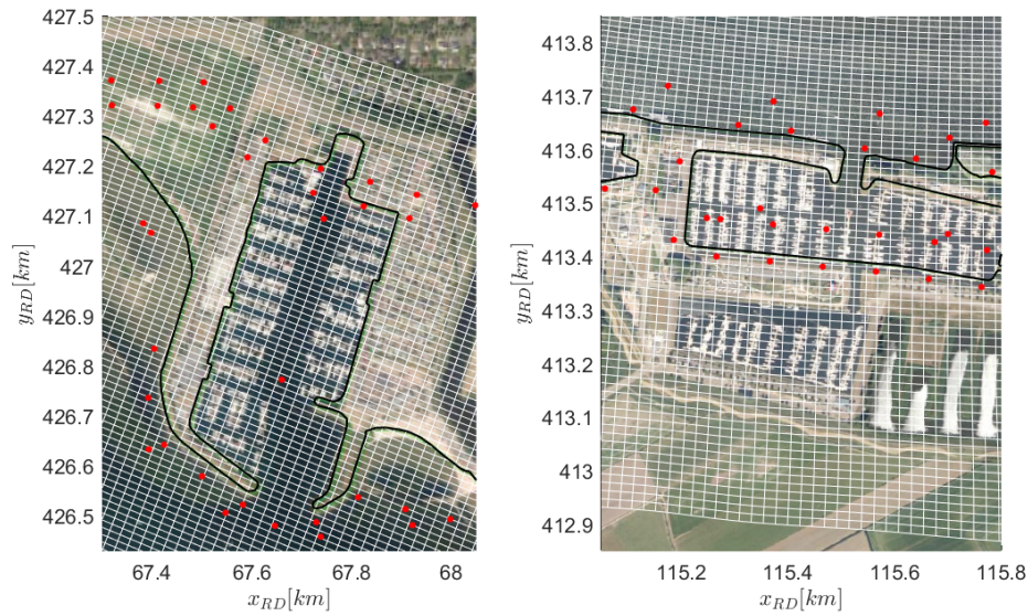
Figure 3.2: Detailed overview of the computation grid at Heliushaven (left panel) and marina Biesbosch (right panel). The red markers represent output locations.
