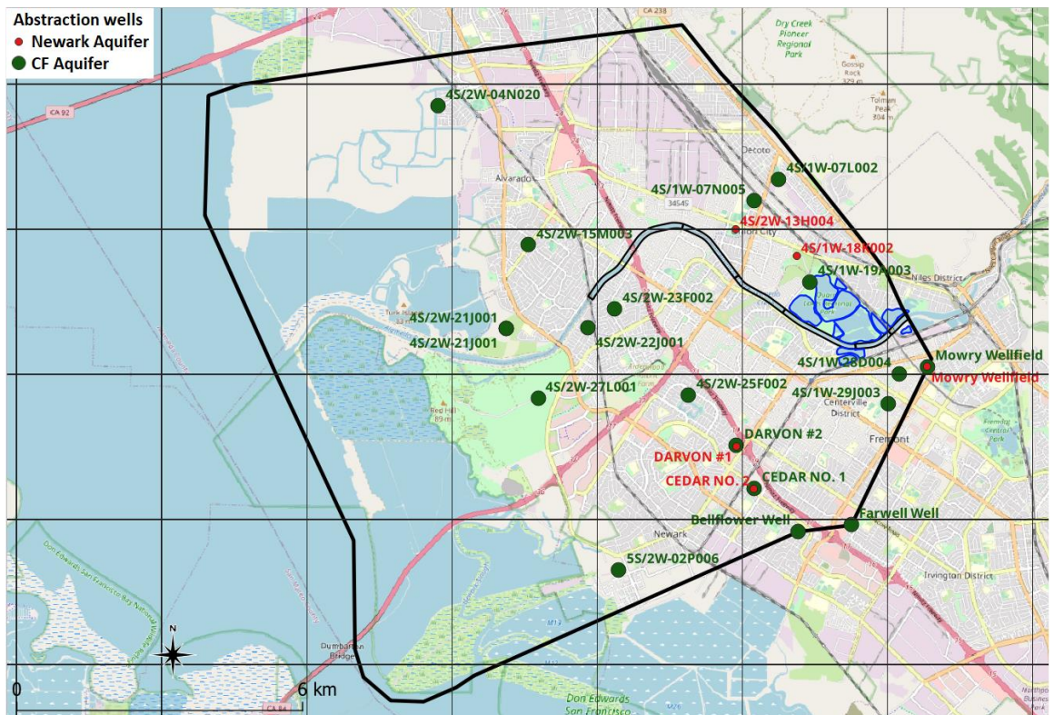
Figure 16 Abstraction wells, as applied in the child model, in the Newark Aquifer (red) and in the Centerville-Fremont Aquifer (green).
