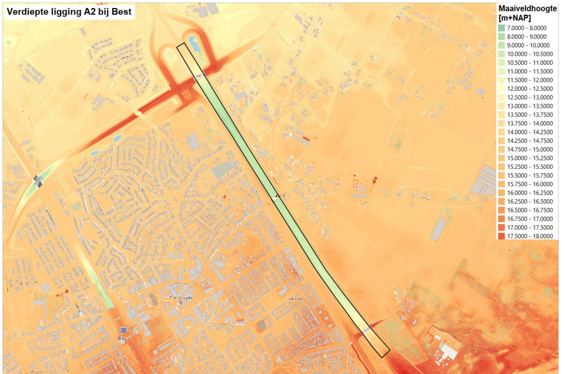
Figure 16 Surface elevation level around the deepened section of highway A2 at Best (source: AHN4)
