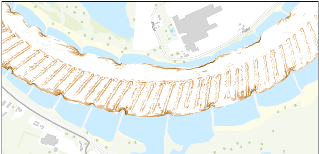
Figure 3.10 Steep slopes (> 6 degrees) around the bottom vanes and groyne tips in the bend at Erlecom on the Waal. From
