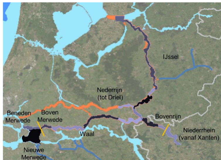
Figure 2.1 Coverage of the sixth-generation hydrodynamic Rhine branches model (orange) and the current DVR instrument (purple areas, the different purple colors indicate the subdomains of which that model consists).
