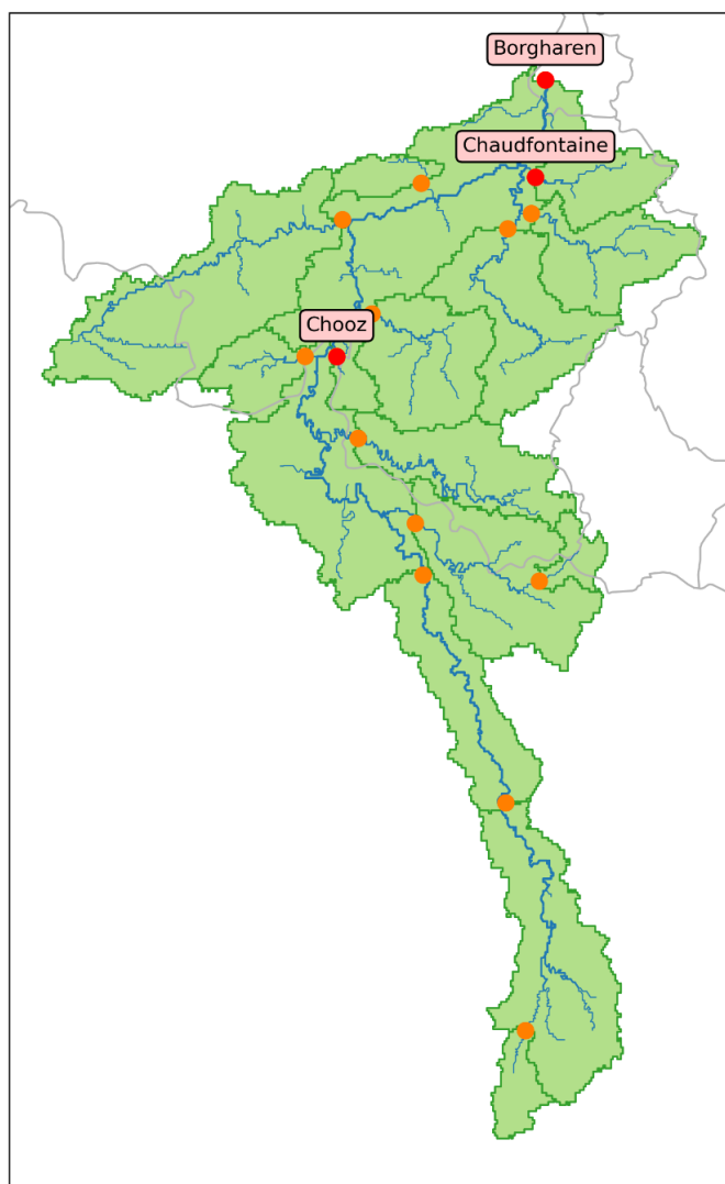
Figure 4-3: Extent of the Meuse model with stations that were analysed in this study. Orange dots present the stations for which simulated discharge time-series can be retrieved. The red dots present the stations for which the results are discussed in the report.
