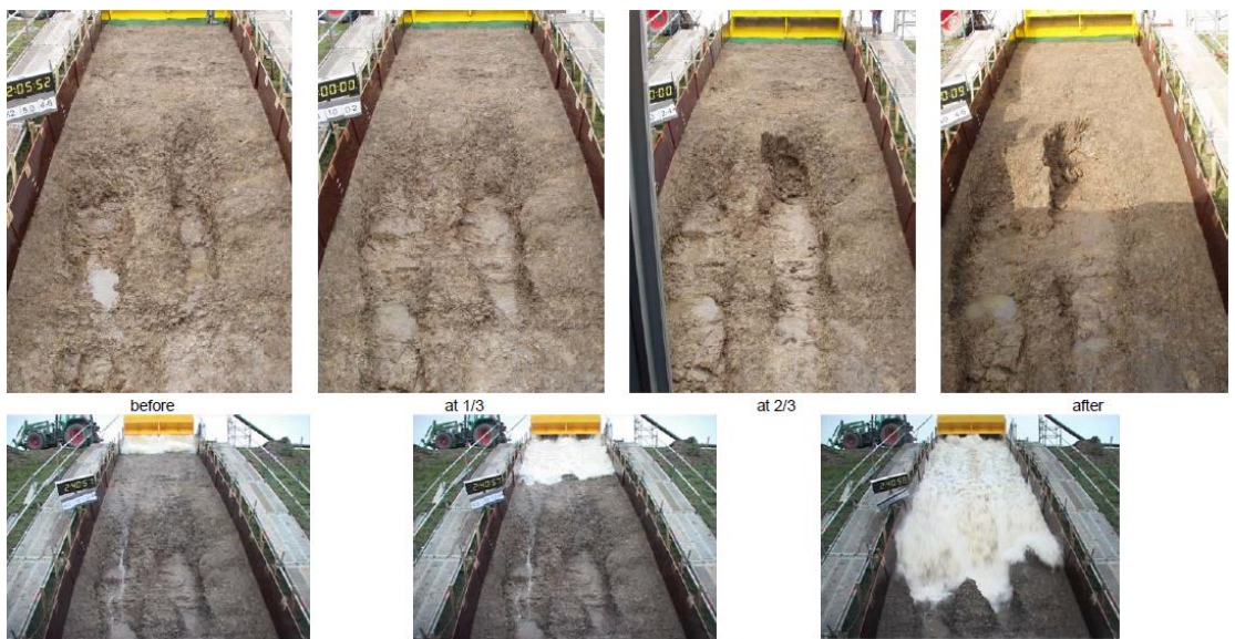
Figure 3.20 Situation during overtopping of 10 l/s/m on bare clay. The biggest wave shown here had a volume of 2.5 m 3 per m width (Akkerman et al., 2007).
