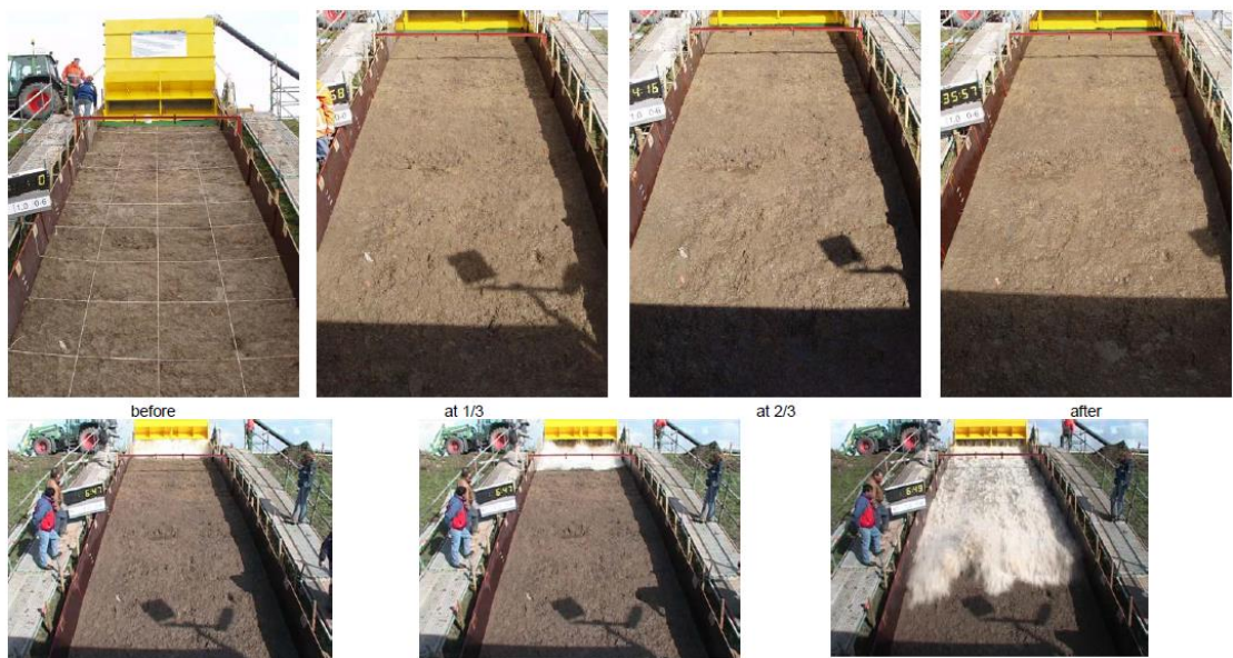
Figure 3.18 Situation during overtopping of 1 l/s/m on bare clay. The biggest wave shown here had a volume of 1 m 3 per m width (Akkerman et al., 2007).
