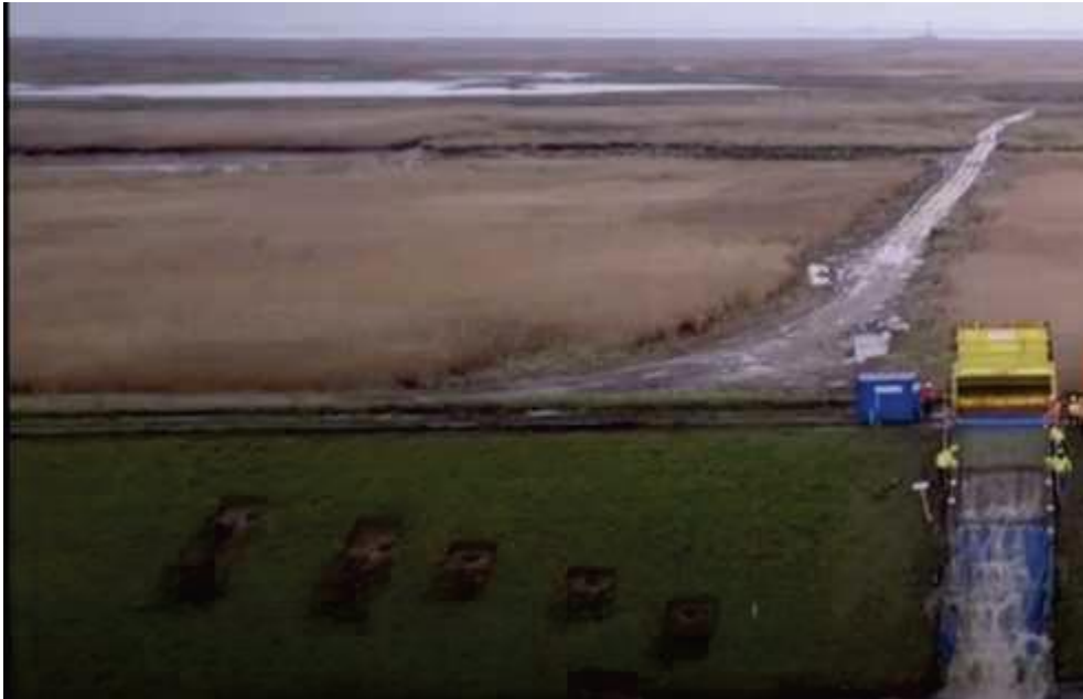
Figure_ D.1.1 Locations where the samples for the EFA tests were taken, visible as holes in the slope to the left of the third wave overtopping tests (Figure 5.5 from Van Damme et al., 2023).
