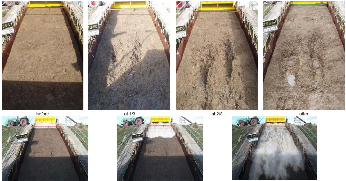
Figure 3.19 Situation during overtopping of 5 l/s/m on bare clay. The biggest wave shown here had a volume of 2.0 m 3 per m width (Akkerman et al., 2007).
