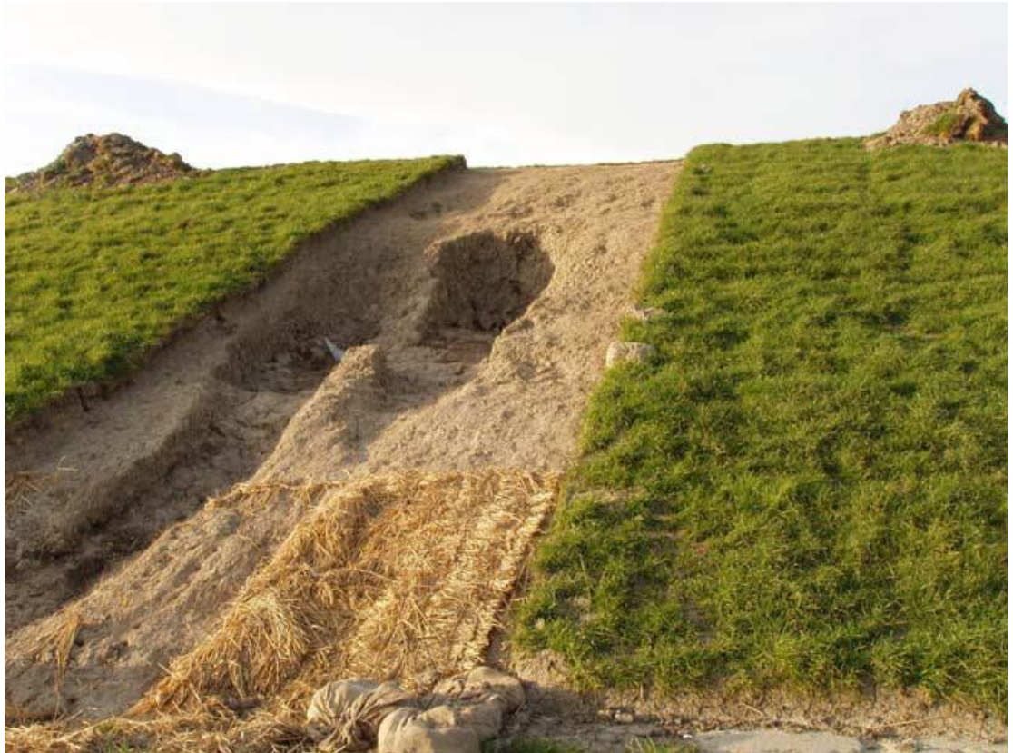
Figure 3.21 Final situation after wave overtopping tests on bare clay and dewatering (Akkerman et al., 2007).
