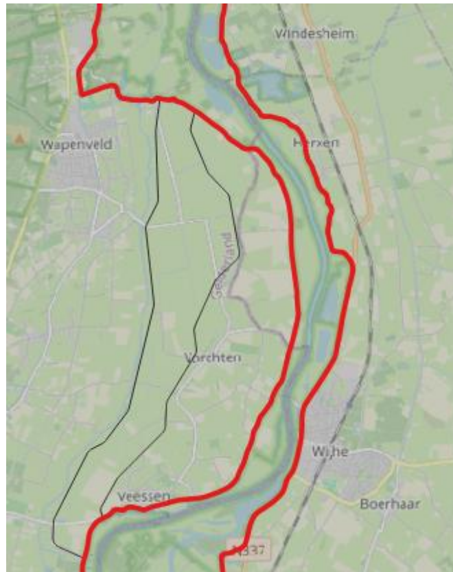
Figure 4.6 Model enclosure (red line) excluding the flood channel Veessen-Wapenveld. The original enclosure including the flood channel is defined by the thin black line.
