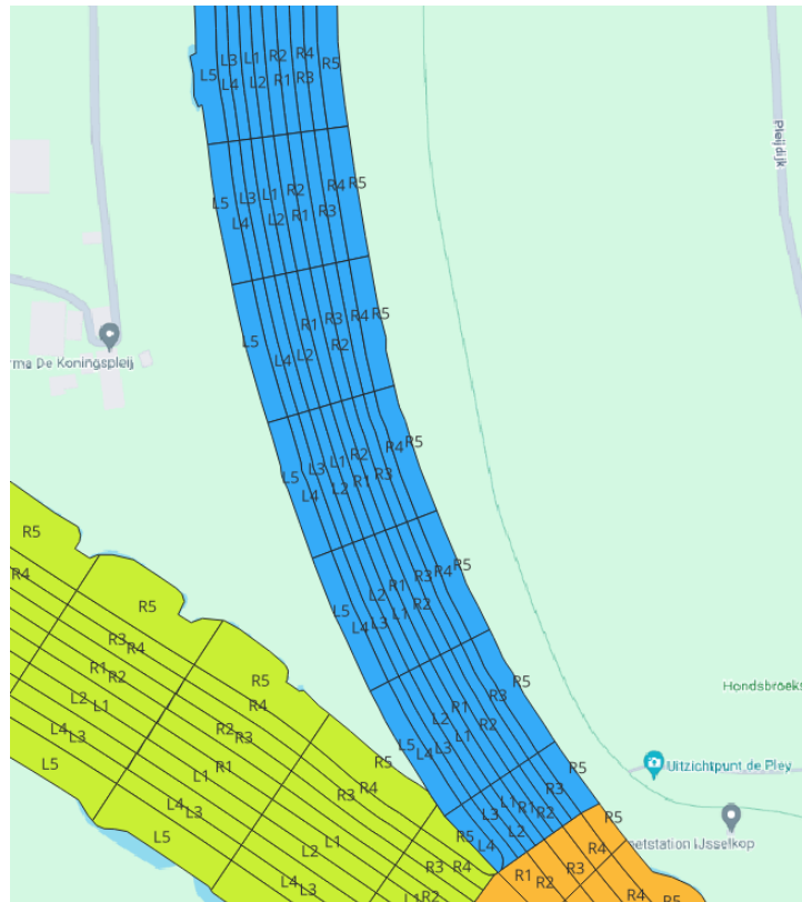
Figure 3.2 Extract from the grid used to analyze bed elevations (from De Joode, 2023).
