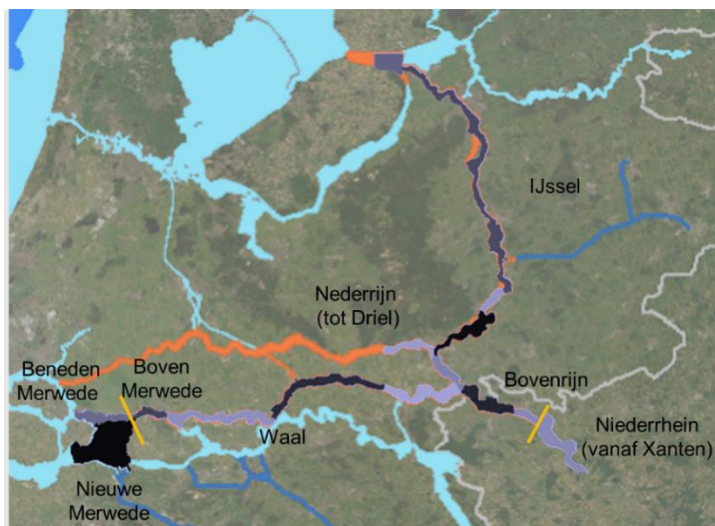
Figure 2.1 Coverage of the sixth-generation hydrodynamic Rhine branches model (orange) and the current DVR instrument (purple areas, the different purple colors indicate the subdomains of which that model consists). Light and dark blue areas are water bodies that are not part of aforementioned models.
