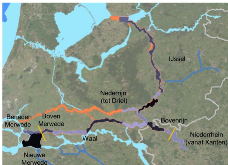
Figure 2.1 Coverage of the sixth-generation hydrodynamic Rhine branches model (orange) and the current DVR instrument (purple areas, the different purple colours indicate the subdomains of which that model consists). Light and dark blue areas are water bodies that are not part of aforementioned models.
