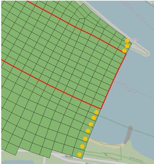
Figure 5.5 Boundary cells excluded from bed level updating (orange dots).
