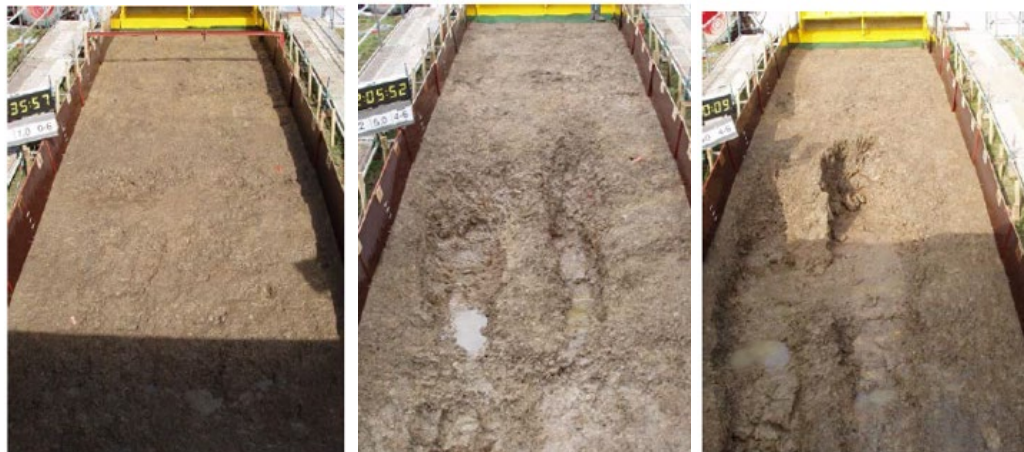
Figure 3.1 Erosion during the Delfzijl tests after 2 hours of 1 l/s/m (left), 6 hours of 5 l/s/m (middle) and 6 hours of 10 l/s/m (right)
