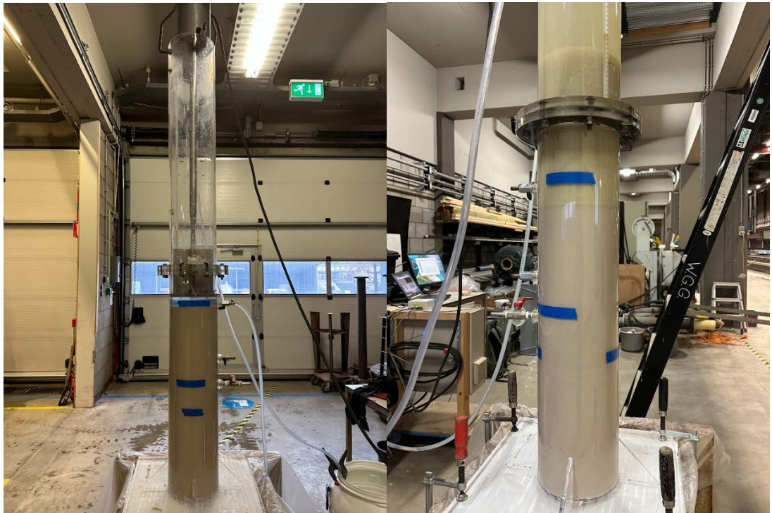
Figure 4-13. The initial setup of the test (based sand layer plus a sand-OCMA bentonite mixture layer of 40 cm - high bentonite concentration) on the left and the final state of the layers after the test on the right.
