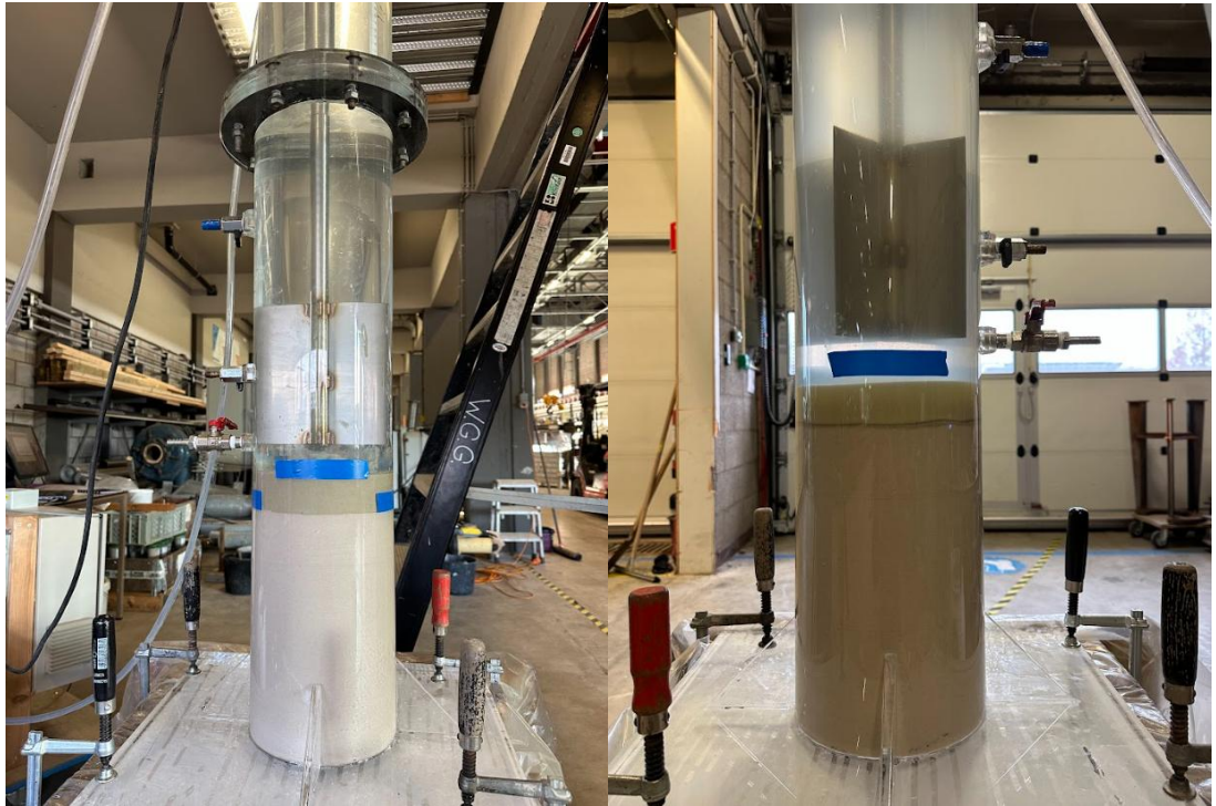
Figure 4-9. The initial setup of the test (based sand layer plus ZBM layer of 4 cm) on the left and the final state of the layers after the test on the right.
