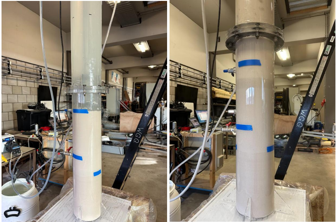
Figure 4-17. The initial setup of the test (based sand layer plus a sand-S1 clay mixture layer of 40 cm - high clay concentration) on the left and the final state of the layers after the test on the right.
