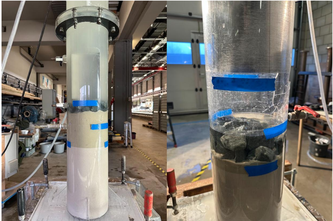
Figure 4-35. The initial setup of the test (an 8 cm premixed ZBM layer in between a 30 cm base sand layer and a 10 cm gravel on top) on the left and the final state of the layers after the test on the right.
