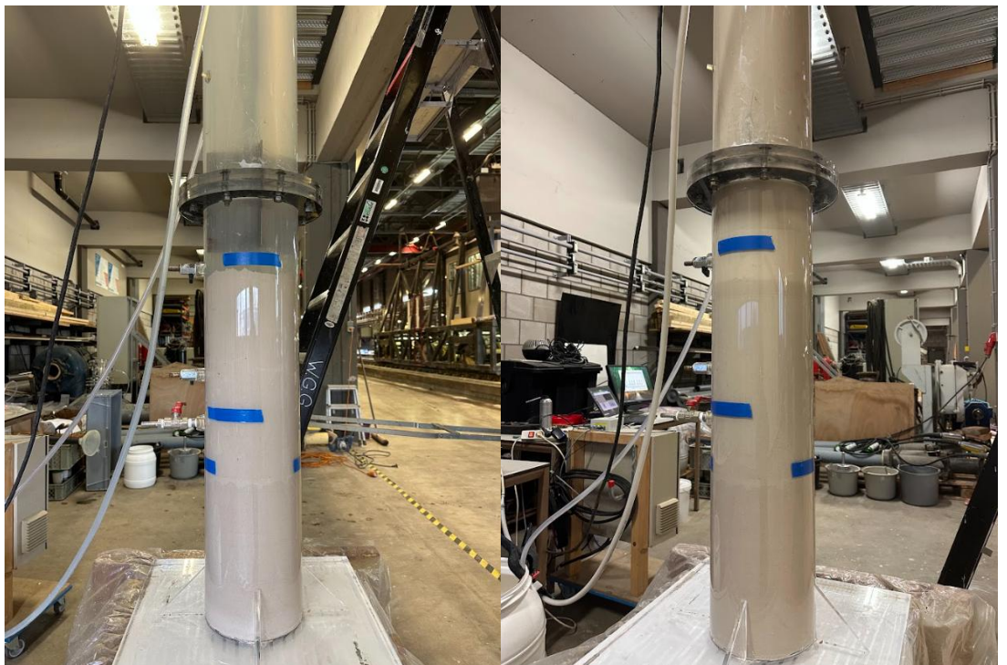
Figure 4-18. The initial setup of the test (based sand layer plus a sand-S1 clay mixture layer of 40 cm - low clay concentration) on the left and the final state of the layers after the test on the right.
