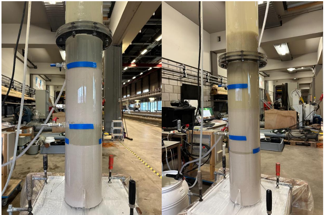
Figure 4-29. The initial setup of the test (an 8 cm premixed ZBM layer in between a 30 cm base sand layer and a 30 cm top sand layer) on the left and the final state of the layers after the test on the right.
