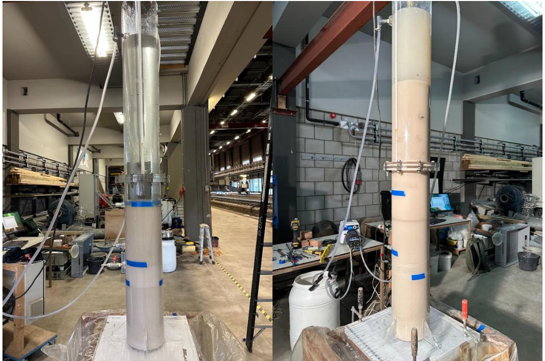
Figure 4-30. The initial setup of the test (a 10 cm S1 clay layer in between a 30 cm base sand layer and a 30 cm top sand layer) on the left and the final state of the layers after the test on the right.
