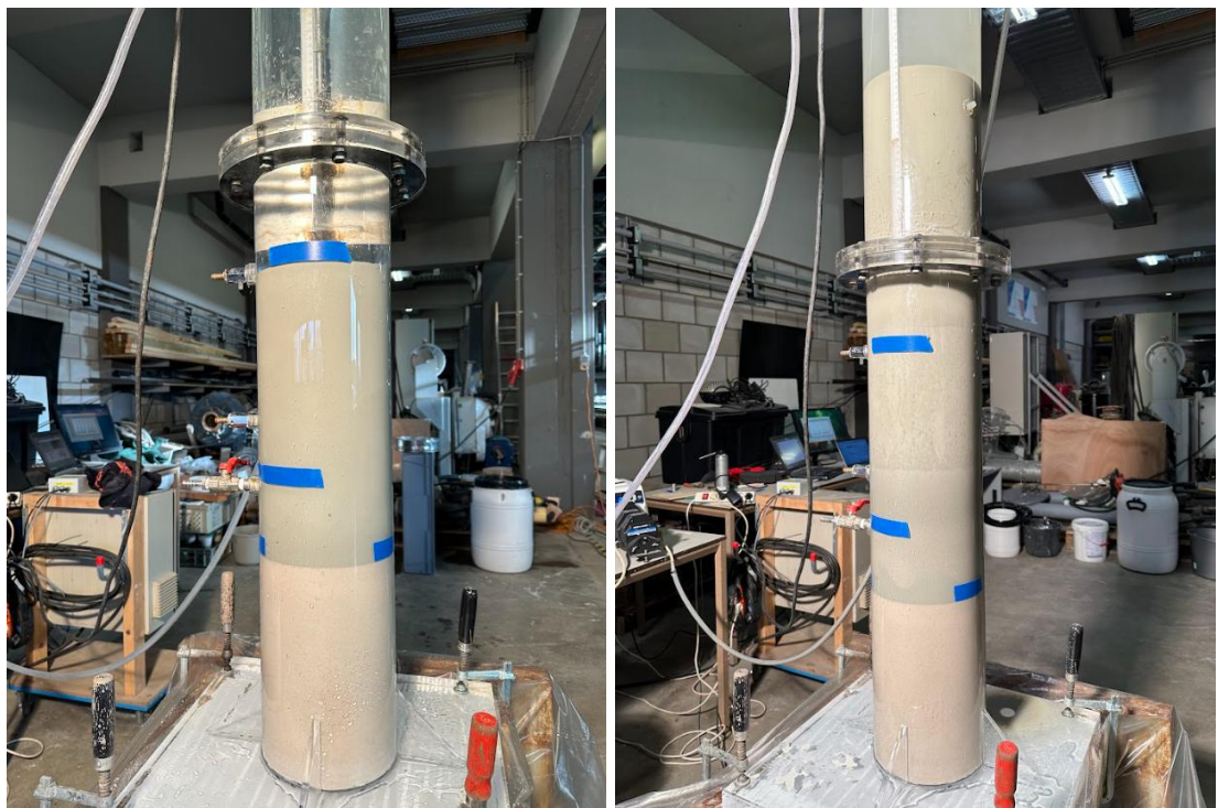
Figure 4-25. The initial setup of the test (based sand layer plus a sand-granulate mixture layer of 40 cm - high granulate concentration) on the left and the final state of the layers after the test on the right.
