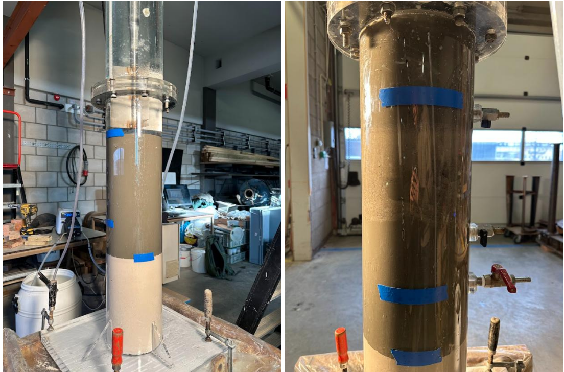
Figure 4-21. The initial setup of the test (based sand layer plus a sand-dredged mud mixture layer of 40 cm - high mud concentration) on the left and the intermediate state of the layers before the test failed on the right.
