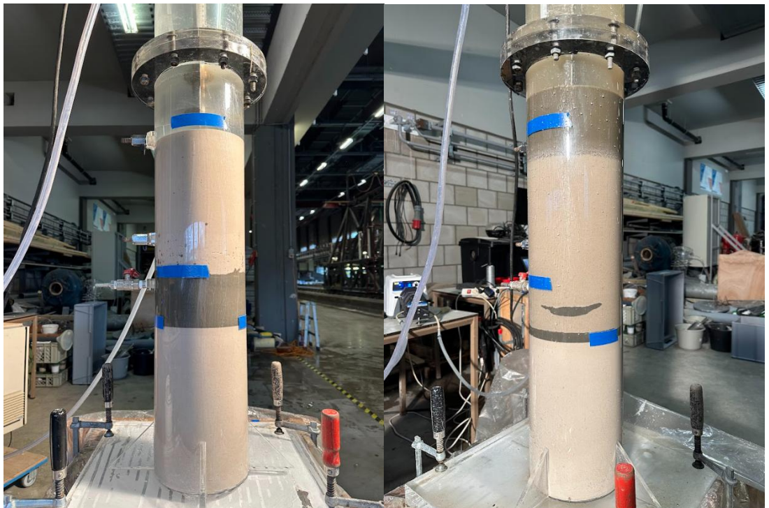
Figure 4-31. The initial setup of the test (a 10 cm dredged mud layer in between a 30 cm base sand layer and a 30 cm top sand layer) on the left and the final state of the layers after the test on the right.
