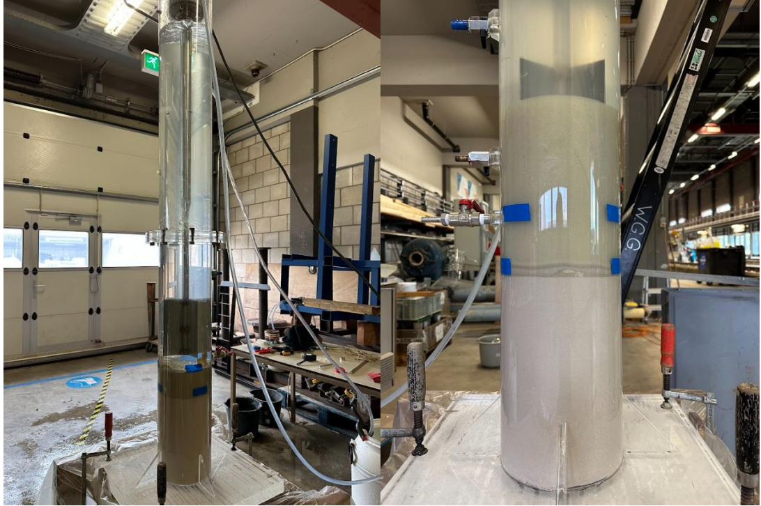
Figure 4-8. The initial setup of the test (based sand layer plus ZBM layer of 8 cm) on the left and the final state of the layers after the test on the right.
