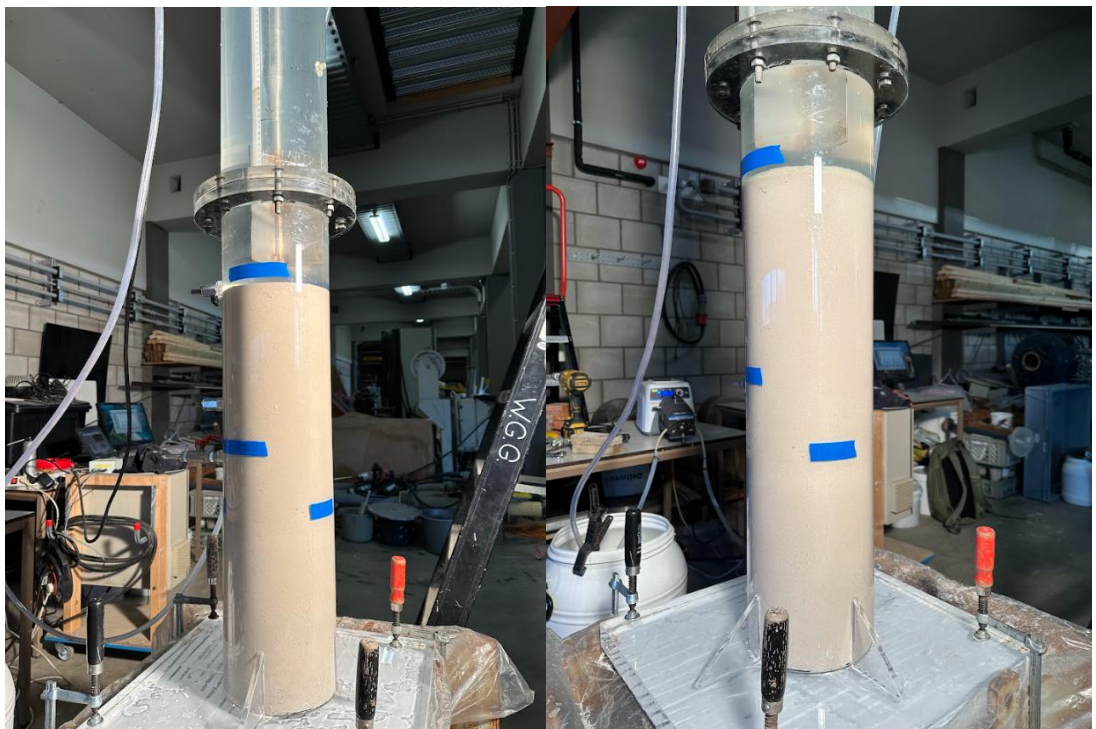
Figure 4-14. The initial setup of the test (based sand layer plus a sand-OCMA bentonite mixture layer of 40 cm - low bentonite concentration) on the left and the final state of the layers after the test on the right.
