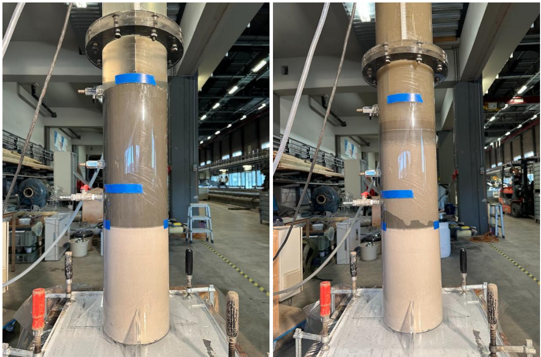
Figure 4-22. The initial setup of the test (based sand layer plus a sand-dredged mud mixture layer of 40 cm - low mud concentration) on the left and the final state of the layers after the test on the right.
