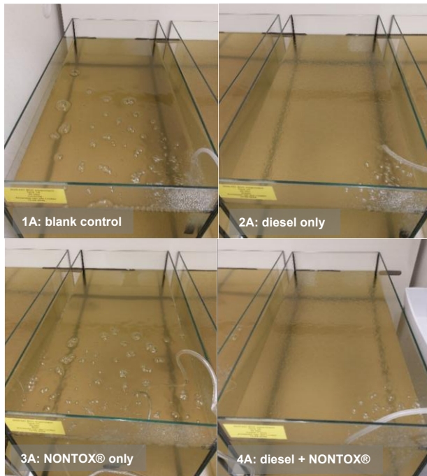
Figure 3-7 Initial setup of aquaria at the start of the experiment, following the addition of diesel to aquaria 2 and 4. Displayed here are the A replicates in clockwise order starting from the top left corner as follows: (1) blank control; (2) diesel pollutant only, (3) NONTOX® treatment only, (4) diesel pollutant and NONTOX® treatment. Note the floating diesel film at the water surface in aquaria 2 and 4.
