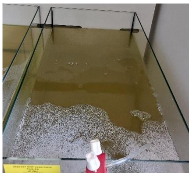
Figure 3-6 Example of the foam formation after NONTOX® treatment to aquarium 4B as generally observed.
