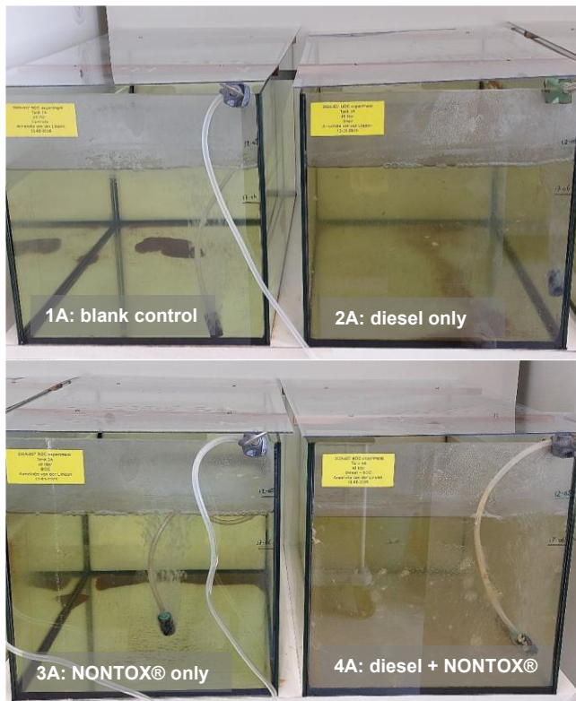
Figure 3-10 Visual differences between the aquaria after 30 days. Displayed here are the A replicates in clockwise order starting from the top left corner as follows: (1) blank control; (2) diesel pollutant only, (3) NONTOX® treatment only, (4) diesel pollutant and NONTOX® treatment.
