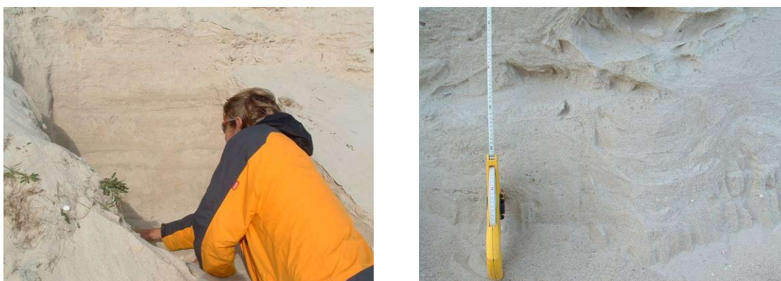
Photo 2.3 Two photos showing convolute bed layers in Plouescat, France (Photos taken by Deltares, 2008).
