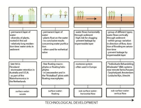
Figure 1: overview of different constructed wetland types and their characteristics. The different types are sorted according to technological development. (based on Fonder and Headley, 2010)
