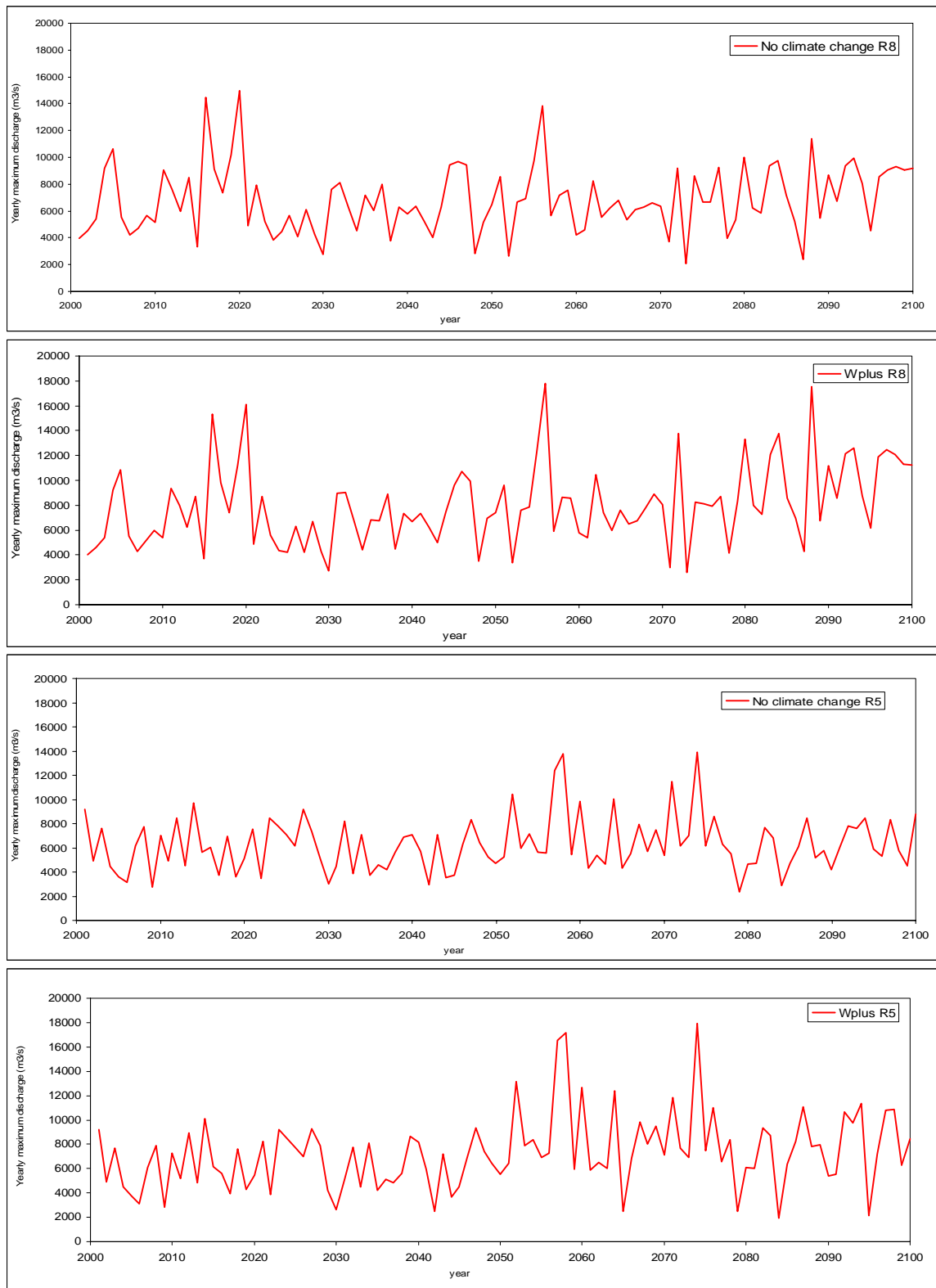
Figure 2: Transient scenarios for two different climate realisations (indicated with realisations 5 and 8) for a situation without climate change and a situations with climate change according to the Wplus scenarios. In 1995 people were evacuated in the Betuwe area when the Rhine discharge was about 12000 m³/s.
